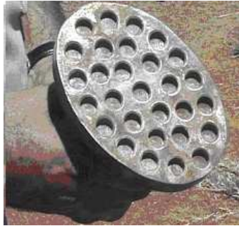
(a) The anvil of the dimple gauge
