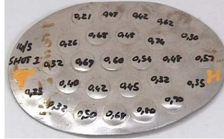
(b) Plate after experiments. The numbers written on the dimples are mm of deflection.
