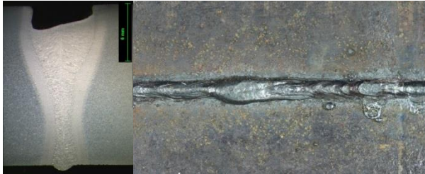
Figure 10: Macrograph and picture of root at 8.2 kW laser power and 7.4 kW arc power (WFS 12 m/min)
