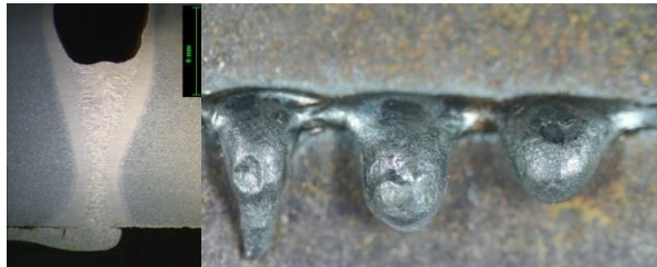
Figure 7: Macrograph and picture of root at 7.7 kW laser power and 7.4 kW arc power (WFS 12 m/min)
