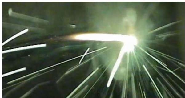
Figure 11: Root formation at 7.7 kW of laser power and 12.1 kW arc power (WFS 20 m/min)
