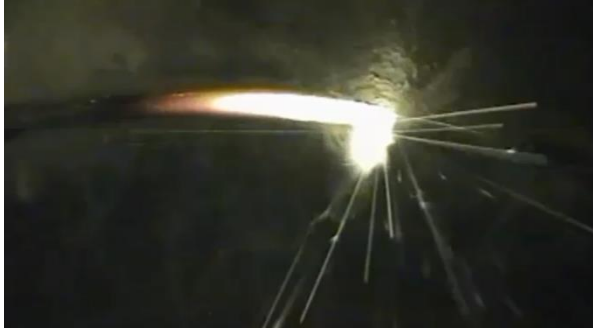
Figure 9: Root formation at 8.2 kW of laser power and 7.4 kW arc power (WFS 12 m/min)
