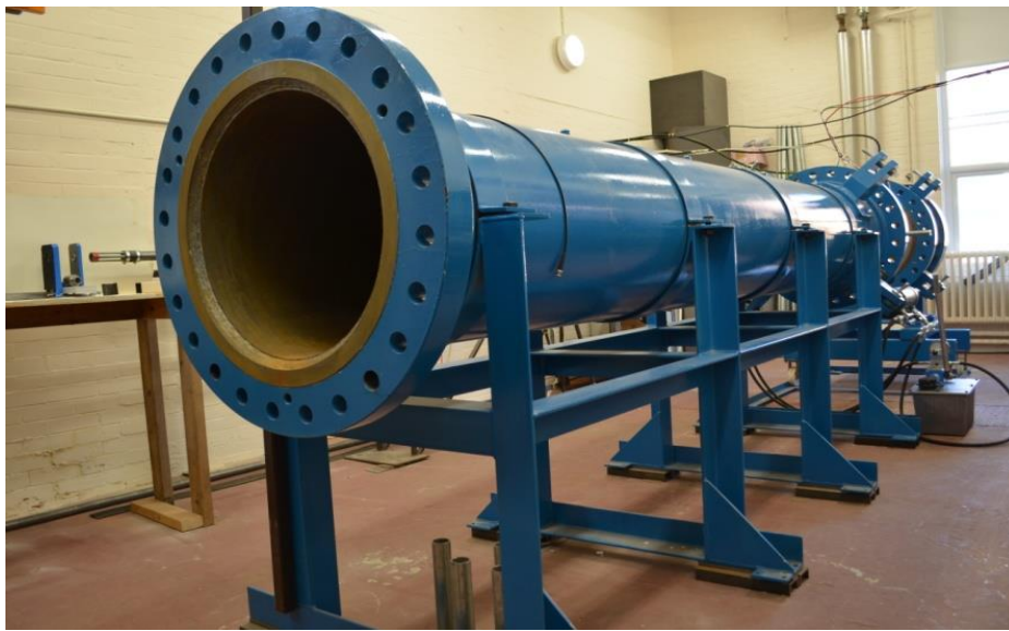
Figure 5. The shock tube used to provide blast loading
