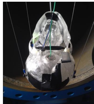
Figure 4. Head simulant suspended in the shock tube
