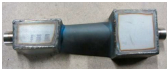
7 The boxes fitted the blade root and shroud to the blades' modified cooling air supply and partial exit, respectively. The blade root (cooling air inlet) is to the right. The blade shroud (main cooling air exit) is to the left
