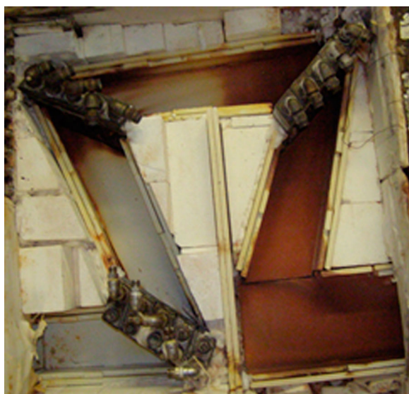
13 Photograph of the cascade gas path after the 1000 h trial showing the development of red/brown discoloration between the second and third cascade stages
