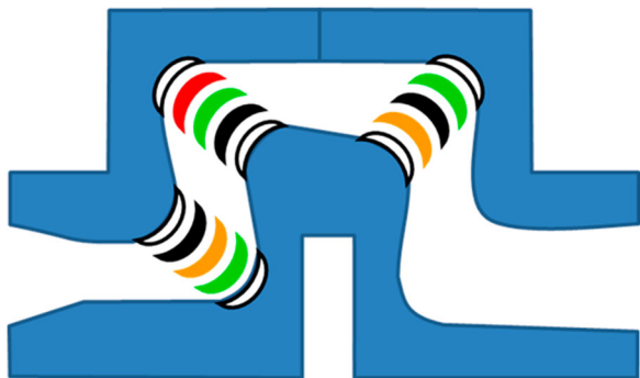
9 Four different TBC coating systems (ceramic and bond coat combinations, indicated by different colours) were applied to blades in the centre of each cascade stage. The blades that formed the cascade walls in each cascade stage (shown in black-and-white) were coated with just the metallic corrosion-resistant coating Sicoat 2464
