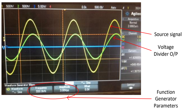
Figure 4.14 Test Signal for Close circuit
