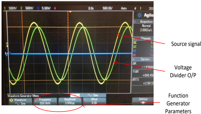
Figure 4.13. Test Signal of Open Circuit
