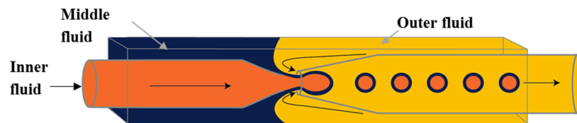
Figure 13. Schematic illustration of coaxial microcapillary fluidic device for making double emulsions in a single step. The geometry requires the outer fluid to be immiscible with the middle fluid and the middle fluid to be in turn immiscible with the inner fluid [14].
