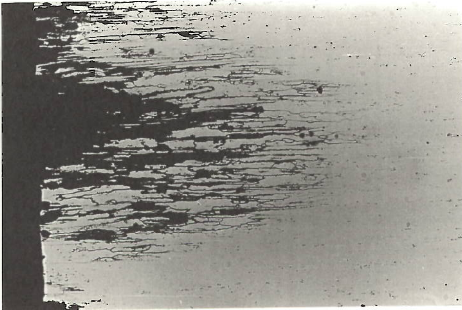
Figure 6.3. : Cross - section showing end grain attack for 2024 after 2000 hours (X50).
