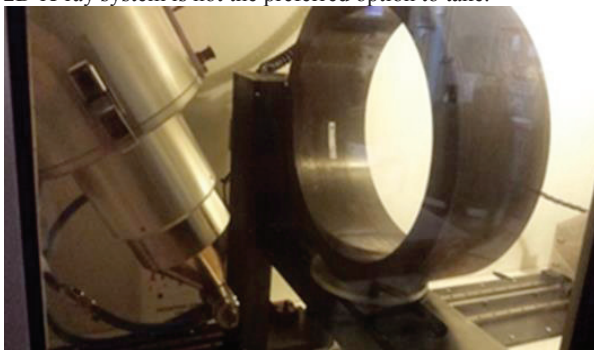
Fig. 7. Experimental set-up of a 2D X-ray system.
