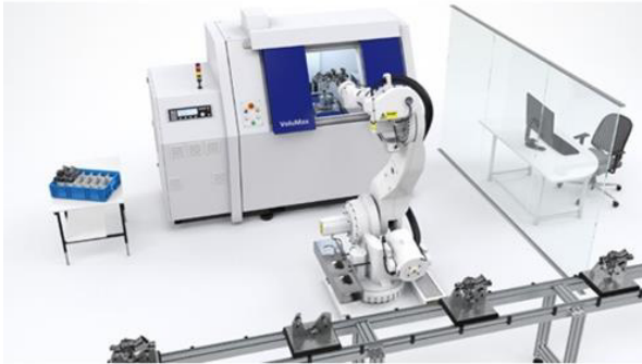
Fig. 13. Fully automated in-line CT system. [19]
