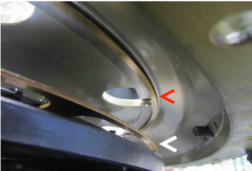
Figure 10. Coils in position before rejoining top cover (static coil red arrow, moving coil white arrow)
