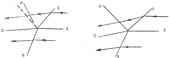
Further increase in the strength of i produces the strong type of transmitted shock t with subsonic flow behind it.
