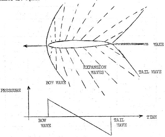
The magnitude of the pressure discontinuity,  $^{(12)}$   $\Delta$  p, across the bow wave, at a normal distance y from a parabolic shaped body of revolution of fineness ratio  $\delta$  and length  $\ell$ , moving through a uniform atmosphere of pressure p at a Mach number M is
