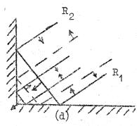
An estimate of the strength, on the basis of the method discussed in section 3, could be obtained as follows. From Table 1  $\Delta$  p  $\gtrsim$  1 lb./sq.ft. Since M is less than 1.4 multiply by 2 and to allow for atmospheric effects multiply by 5. Hence  $\Delta$  p = 10lb./sq.ft.
