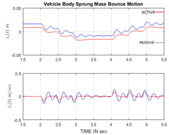
Figure 5. Without Preview: Vehicle Sprung Mass Characteristics (Passive and Active Suspension).
