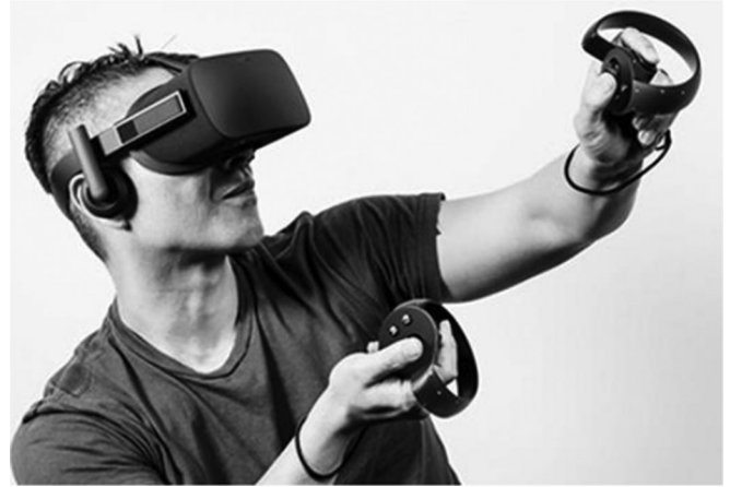
Fig. 3. Oculus Rift system, showing the immersive HMD with headphones, and the Oculus Touch input interface.
