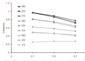
Fig 4. Effects of inter-aperture clutter motion on interferometric direct volume coherence by polarimetric channel. RMS wheat ear displacements are zero (top 3 curves), 0.7cm (middle 3) and 1.3cm (lower 3). VV returns come predominantly from the top of the canopy where displacements are greatest.
