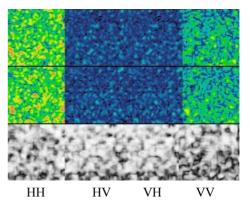
Figure 3. Simulated GB-SAR images of wheat for the 20cm baseline with no clutter motion and the resulting coherence image formed using a 5 by 5 window.
