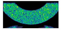
Fig. 6. Simulated static-case GB-SAR image using the distributed point scatterer model, for the parameters described in the preceding text. The image represents an area 20m in azimuth and 10m in ground-range. The features at the bottom corners are associated with range-ambiguity aliasing.
