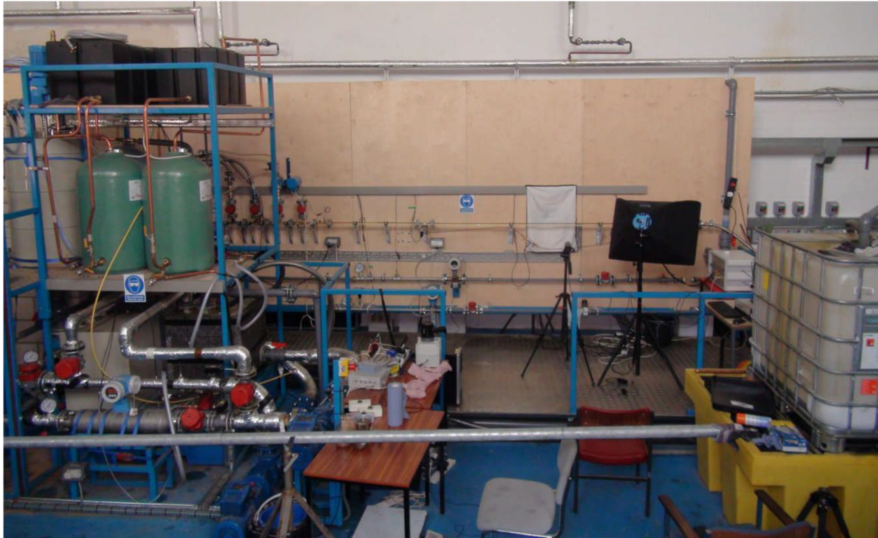
Figure 3-8: Pictorial view of 1-inch four phase transport facility at Cranfield University PASE laboratory
