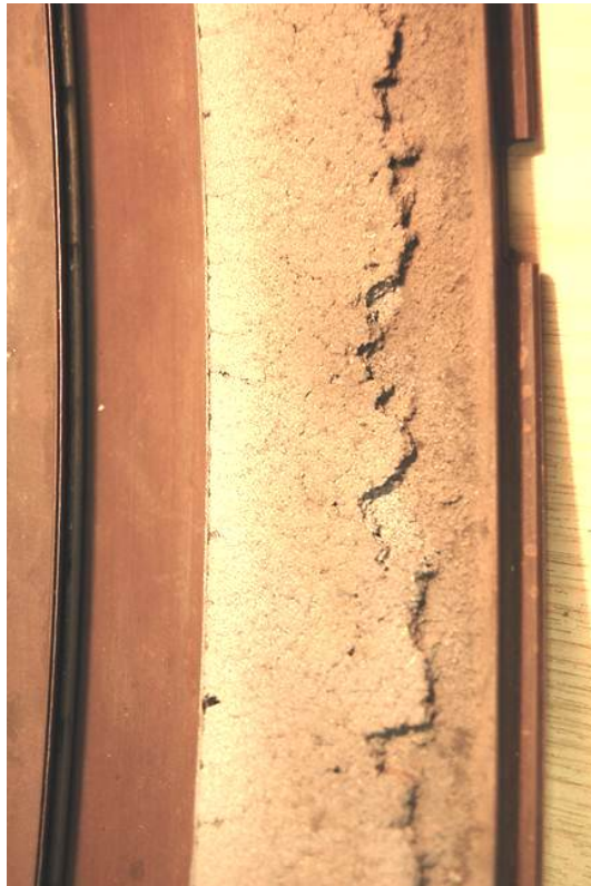
(b) Service Failure - Mudflat Cracking and Delamination
