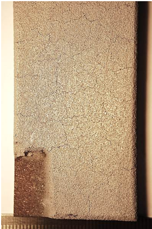
(c) Mudflat Cracking on a Test sample in the Laboratory
