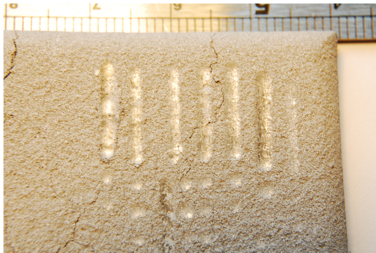
Figure 10.25: Surface of an Abradable Sample after Scratch and Indentation Testing
