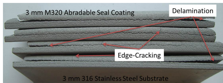
(a) Delamination of the Abradable during Heat-Cycling
