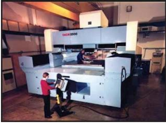
Figure 2-7 left: The Kodak OAGM 2500 built by Cranfield Precision (source: http://cranfield-precision.blogspot.co.uk/2011/10/kodak-oagm-2500-off-axis-grinding.html ); right The BoX machine at Cranfield University (source: [79]).
