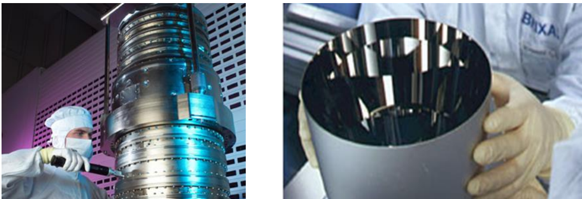
Figure 2-5 Extreme Ultraviolet lithography: the 193 nm lithography system Starlith1700 (left) and the next generation EUV mirror (right). Source: [45].
