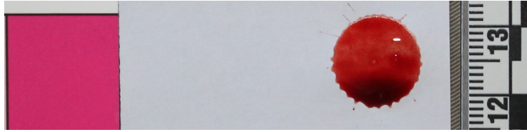
(b) The accepted bloodstain resulting from a droplet with d_0 = 3.13 \times 10^{-3} m and u_0 = 4.85 \text{ m s}^{-1} . The outer diameter is d_{\text{out}} = 1.42 \times 10^{-2} m.
