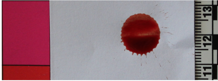
(a) The omitted bloodstain resulting from a droplet with d_0 = 3.22 \times 10^{-3} m and u_0 = 4.88 \text{ m s}^{-1} . The outer diameter is d_{\text{out}} = 2.89 \times 10^{-2} m.
