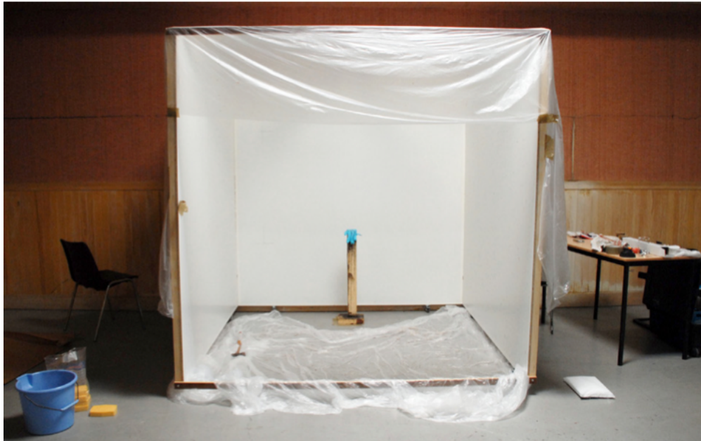
Figure 2.20: Experimental set up by Maloney et al. [2011b] where a pool of blood sitting on a hockey puck is struck with a hammer.
