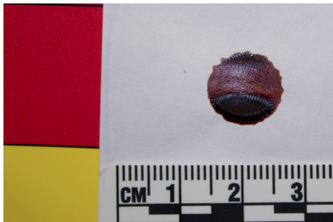
Figure 3.2: Photograph of the resulting bloodstain from a horse blood droplet, of radius 2.3 \times 10^{-3} m, falling from a height of 0.5 m.
