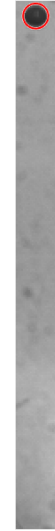
(b) Screenshot from the DVVP showing the program cropping the high-speed video frame and outlining the droplet found.
