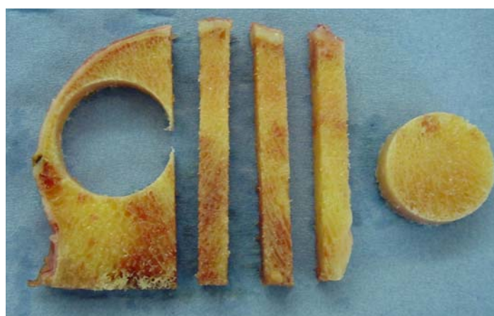
Figure 6.14 Central slice of an osteoarthritic femoral head, with a disk sample and three beam samples taken in the AC direction (Ac: Notch across the trabecular structure)
