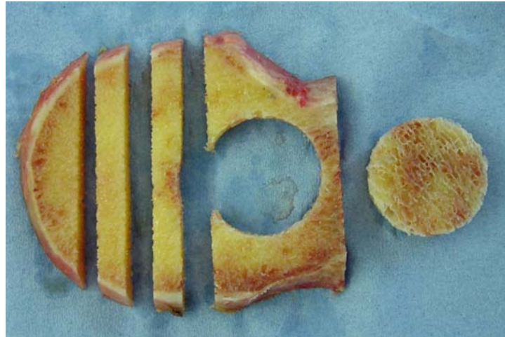
Figure 6.15 Central slice of an osteoarthritic femoral head, with a disk sample and two beam samples taken in the AL direction. (AL: Notch along the trabecular structure).
