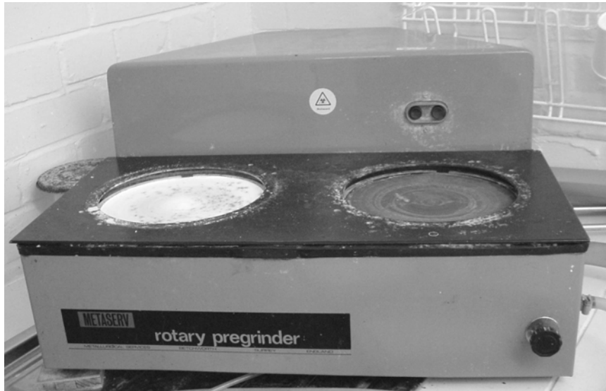
Figure 6.16 The rotary pregrinder used for the grinding of samples to the correct size.
