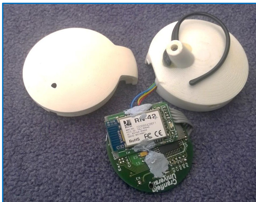
Figure 5-18: The EPMS v2 with its 3D-printed enclosure
