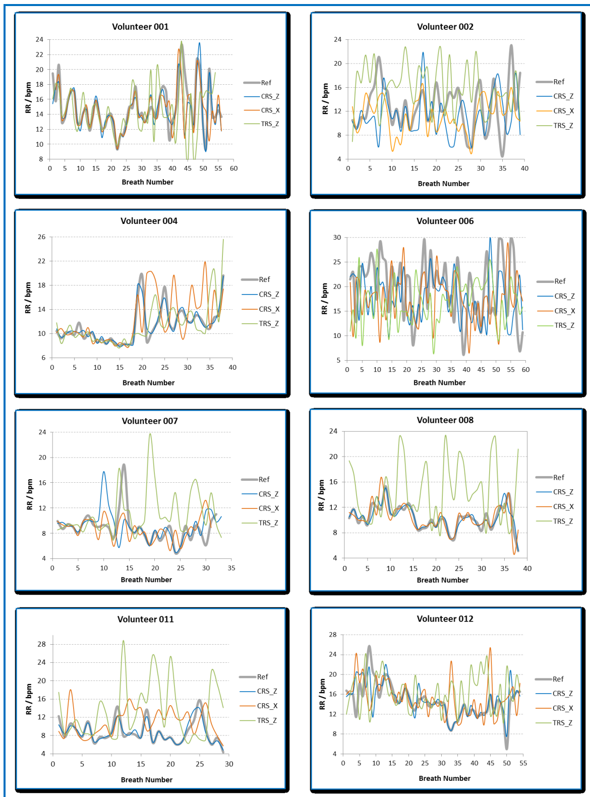
Figure 4-14: A comparative plot of instantaneous breath-by-breath RRs for each of the eight study participants
