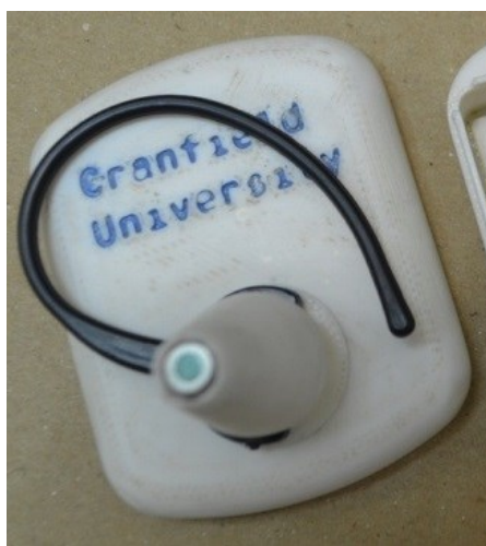
Figure 5-27: A photograph showing the lens of the IR thermometer mounted in the aperture of the EPMS v4 sensor probe
