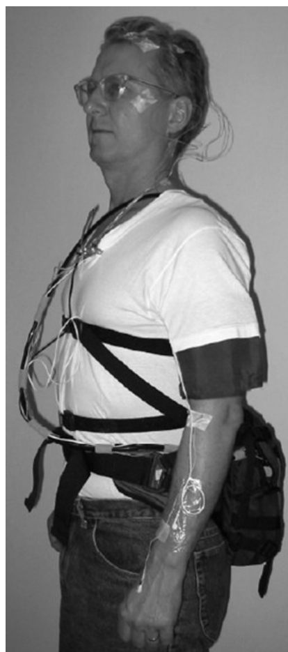
Figure 1-21: An example of an ambulatory physiological monitoring system for EEG, HR, RR, temperature, bioimpedance and BP.
