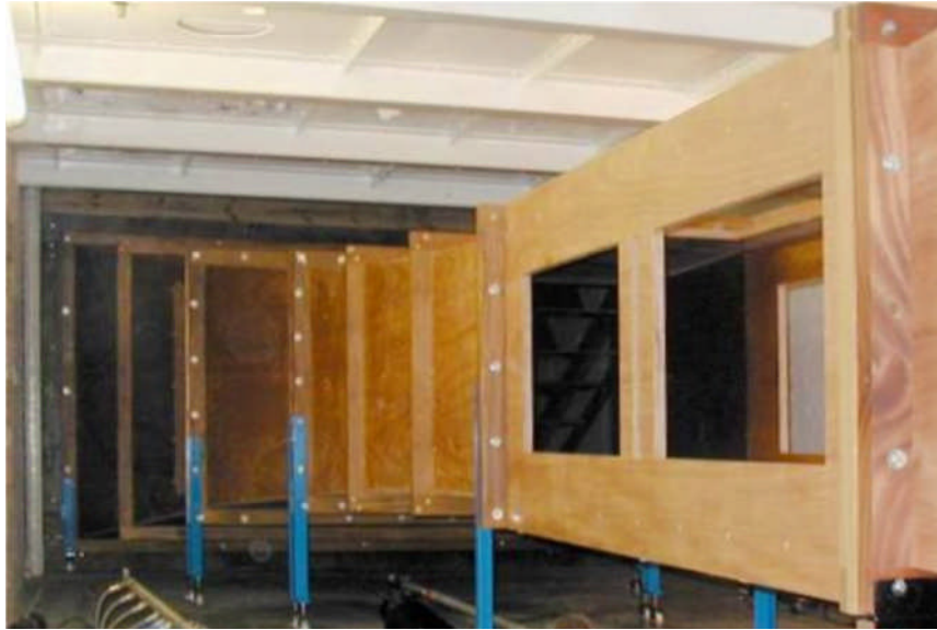
Figure 3-1 Convergent entry (left) to 760mm square working section (right), Luxford (2005)
