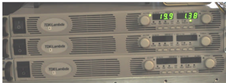
Figure 3-16 Flange preheater controllers
