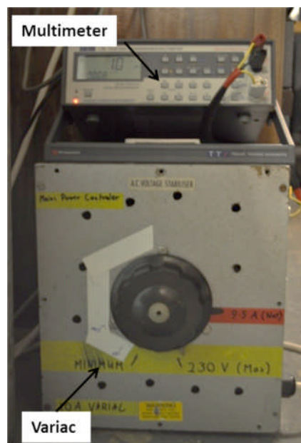
Figure 3-6 Boiler Power Controller (Variac)
