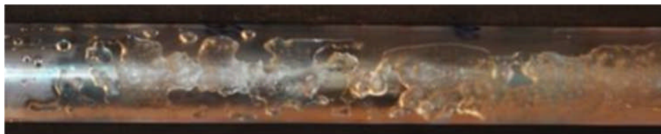
Figure 4-18 Ice layer inside the pipe in Run 22 at the end of the test. The direction of internal airflow is from left to right
