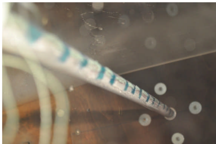
Figure 3-30 Thermocouples embedded in the vertical pipe and fixed with heat resistance self-adhesive tape. (The pipe is installed inside the test section)
