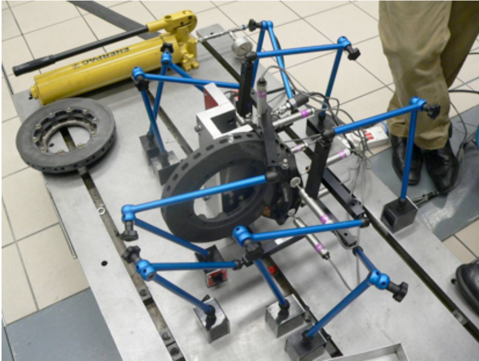
Figure 4-15 : Caliper static deflection test measurements rig
