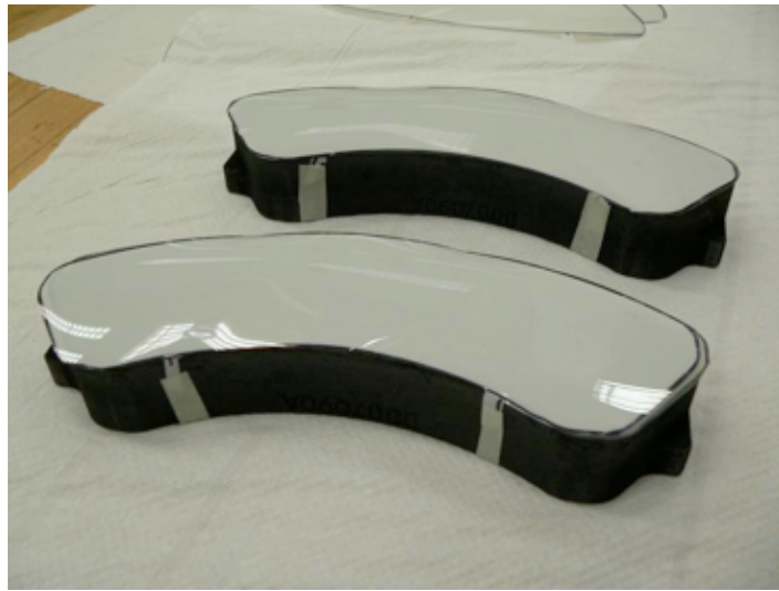
Figure 4-2 : Set of pads with pressure sensitive paper placed on friction surface
