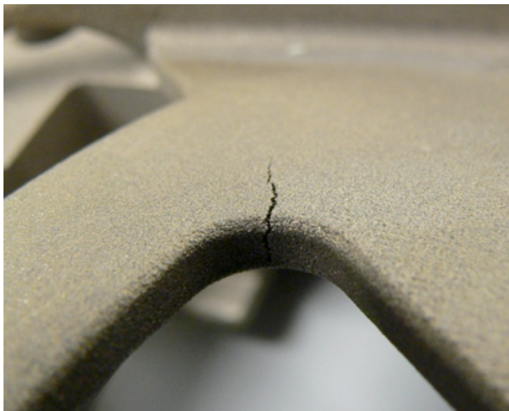
Figure 8-46: SLS model, details of cracks (b)
