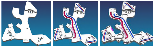
Fig. 56. Top down design of a conventional manifold by starting with the maximum allowed volume (left), removing material for the functional surfaces (center) and then reducing mass (right). Courtesy of ASML.
