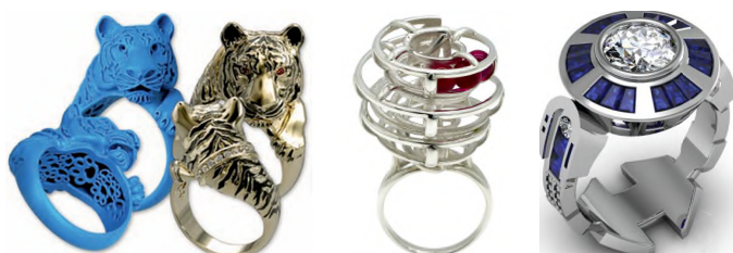
Fig. 9. Jewellery produced with AM: award winning Tiger Ring from OG-Art - pattern printed in wax on a Solidscape machine (via [34]) (left), Kinetic Ring from Vulcan Jewellery (available for purchase) (center, courtesy of Vulcan Jewellery); custom R2D2 inspired ring from Uptown Diamond and Jewellery - pattern printed in wax on a 3D Systems ProJet machine [4] (right).
