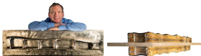
Fig. 45. Ti-6Al-4V wing spars (1.2m long) built back-to-back on a sacrificial build plate for BAE Systems [352]: side view show one wing spar (left) and top view showing both wing spars (right).
