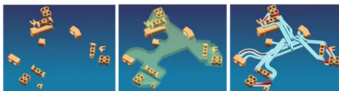
Fig. 57. Manifold designed from the bottom up for AM starting with the interfaces (left), defining the maximum envelope as a constraint (center), and then adding functional features and reinforcement (right). Courtesy of ASML.
