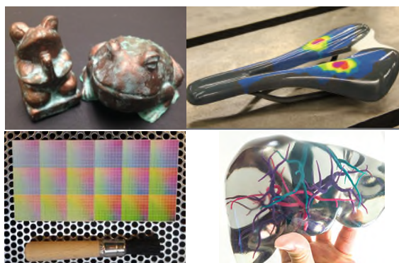
Fig. 8. AM objects in full color: frog and toad models printed using paper-based selective deposition lamination on an Mcor IRIS and colored to appear as aged copper (top left) [215]; bicycle seat colored to show simulated pressure distribution from a rider printed on an Objet Connex3 (top right) [294]; plates showing a 9x9x9 set of color options from a ZCorp ZPrinter 650 before and after brushing (lower left) [92]; and a surgical planning model of a human liver printed on an Objet Connex3 in clear and colored resins [303].
