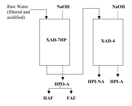
Figure 4.3 Schematic of Fractionation Process
