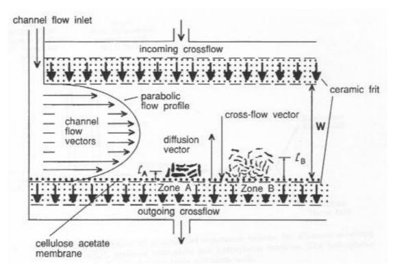
Figure 2.5 Illustration of Flow-Field Flow Fractionation (Beckett et al. 1992)
