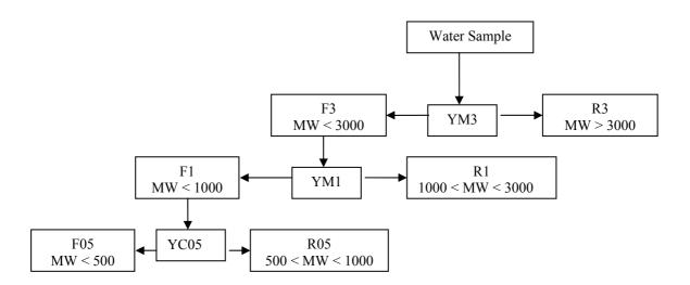
Figure 4.4 Schematised procedure for ultrafiltration fractionation
