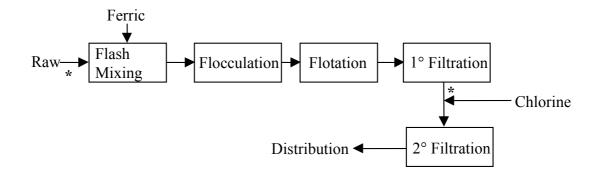
Figure 4.2 Process schematic of Rivington WTW (United Utilities)
