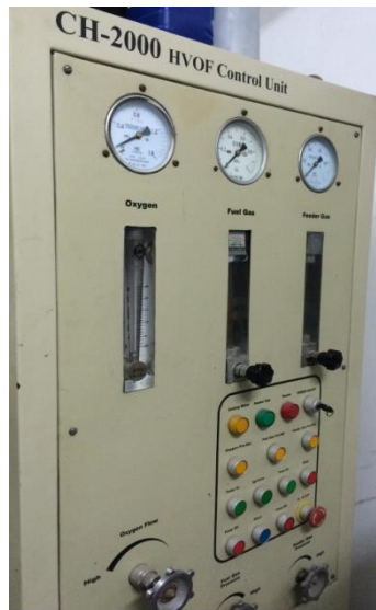
Figure A-6 Oxygen and fuel flow rate controller for CH-2000 torch
