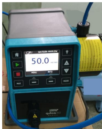
Figure A-7 Liquid feedstock injection pump
