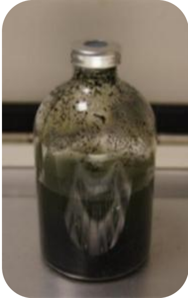
Figure A-4 Biochemical methane potential (BMP) assay consisting of substrate and inoculum (at VS seed :VS substrate ratio of 2:1), deionised water to bring working volume to 60 mL and nutrient stock solution. Samples were incubated in a temperature controlled shaker at 37.5°C ± 0.5 at 150 RPM.
