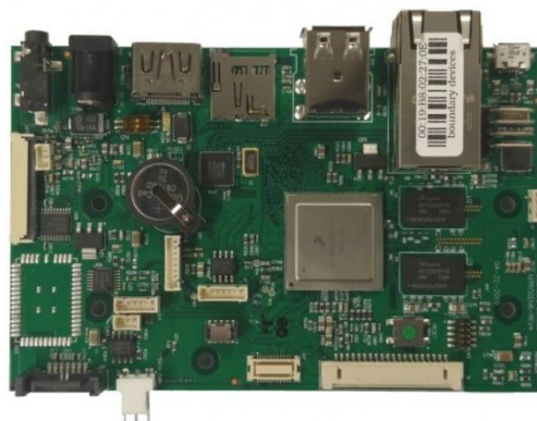
Figure 3-10: Nitrogen 6x embedded board (Boundary Devices, 2012)
