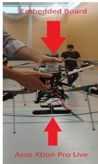
Figure 3-31: Aerial platform & payloads integration
