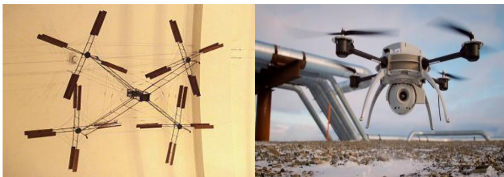
Figure 2-7: [Left] Breguet-Richet Gyroplane No.1, 1907 [Right] Quadrotor (Devaud et al., 2012)
