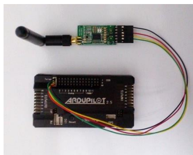
Figure 3-17: XBee & APM hardware interface (ArduPilot, 2013)
