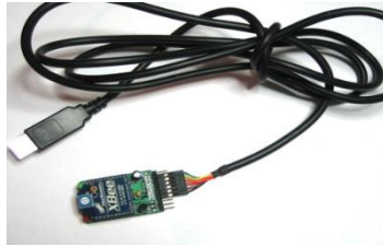
Figure 3-20: Xbee module & FTDI cable for interface with the PC
