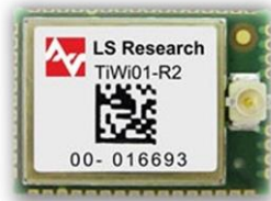
Figure 3-11: Nitrogen 6X Add-on Ti-Wi Module (Boundary Devices, 2012)
