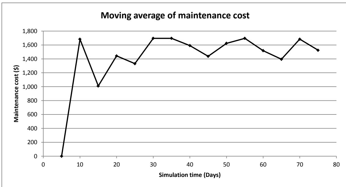
Figure 6-14 Warm-up analysis for case A simulation model considering maintenance cost as an objective
