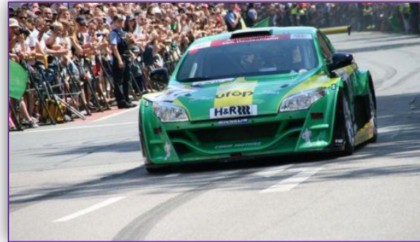
Figure 2-14: Four Motors GmbH green racer; the body-shell is made of plant fibre reinforced composites
