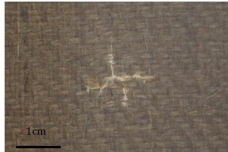
Figure 5-6: Fractographs of the samples subjected to gas gun impact testing at 20m/sec
