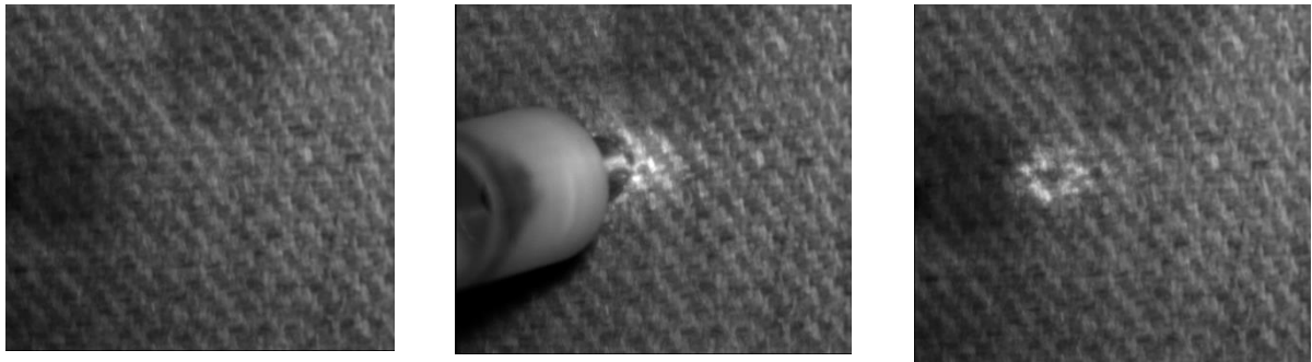
Figure 4-7: Impact sequence for the 23m/sec test of flax/PLA samples (high speed camera imaging)
