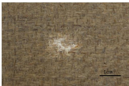
Figure 5-7: Fractographs of the samples subjected to gas gun impact testing at different temperatures
