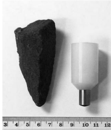
Figure 4-2: Road stone, projectile and impactor [80]
