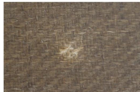
Figure 5-7: Fractographs of the samples subjected to gas gun impact testing at different temperatures
