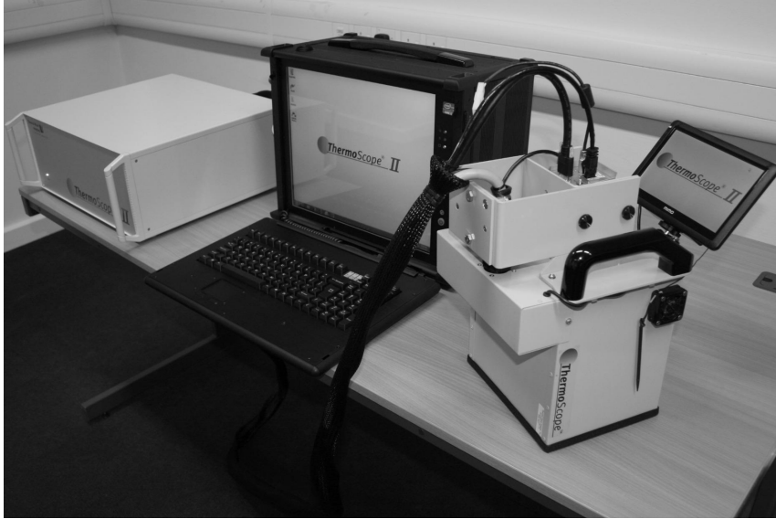
FIGURE 5.21: Components of thermography system ThermoScope II (Widjanarko et al., 2012).
