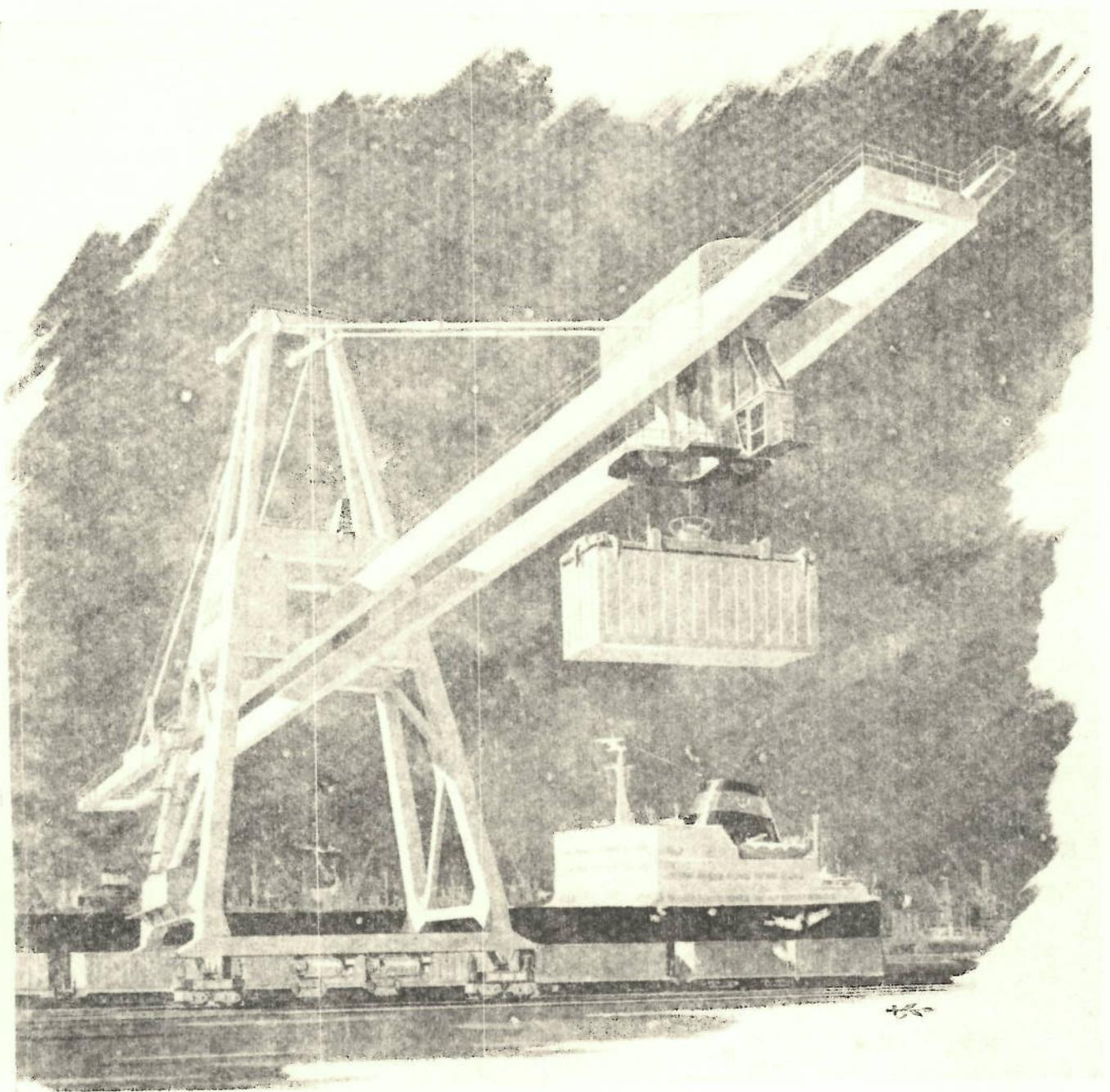
Fig. 3 Container crane of the type installed at Churchill Dock, Antwerp.
