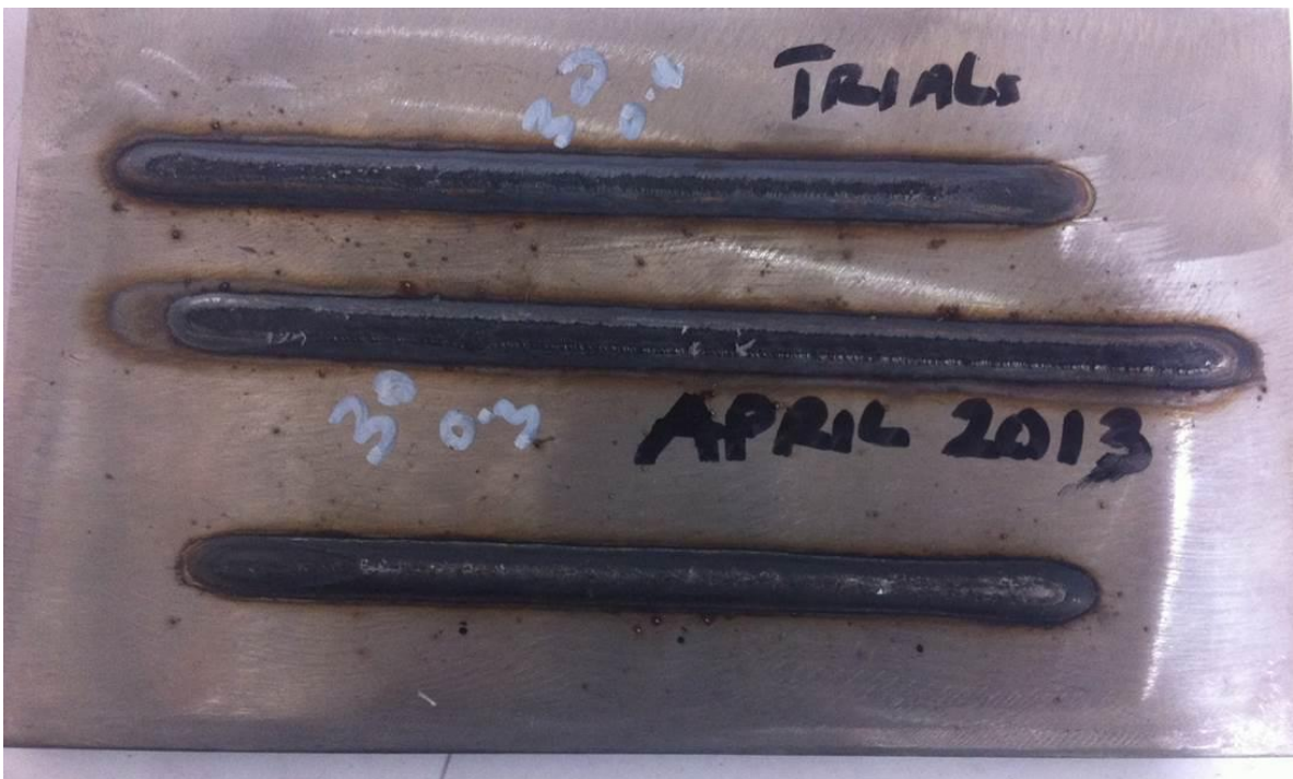
Figure 4-2: Trial made on austenitic stainless steel plate
