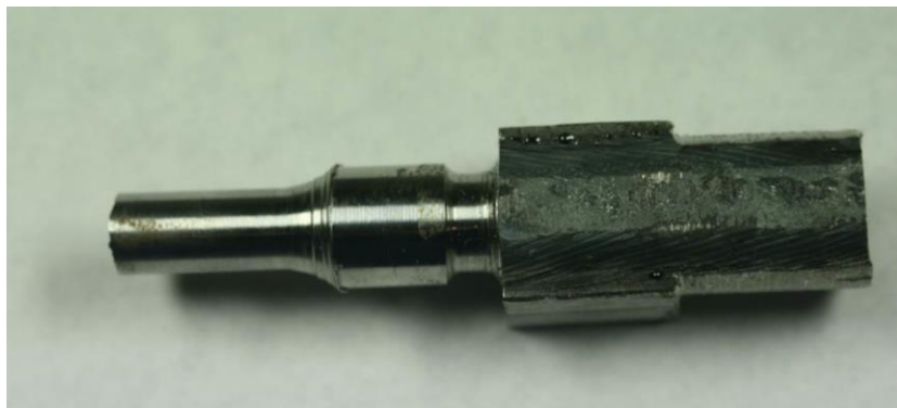
Figure 3-9: Machined and tensile tested sample
