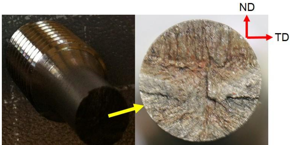
Figure 3-35: Macrostructure of the cross section of fractured tensile sample (post weld cold rolled sample)
