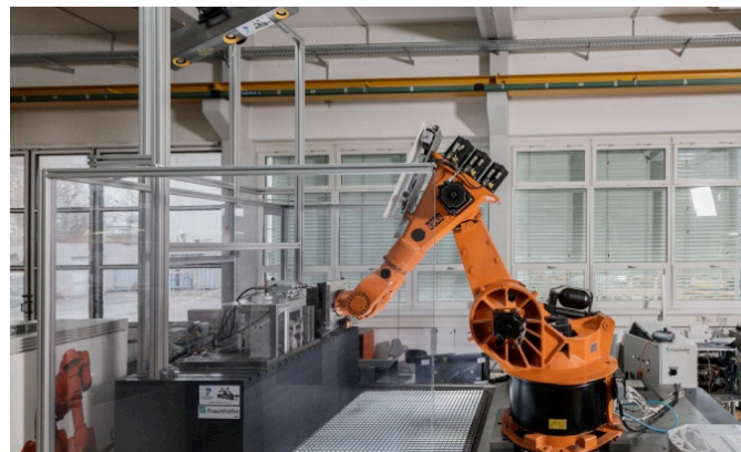
Figure 1: Robotic machining cell with K600 measurement system, Chopper 3300 spindle and KR125 robot.
