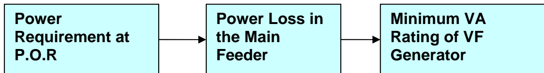
Figure 7-2 Minimum VA Rating of VF Generator
