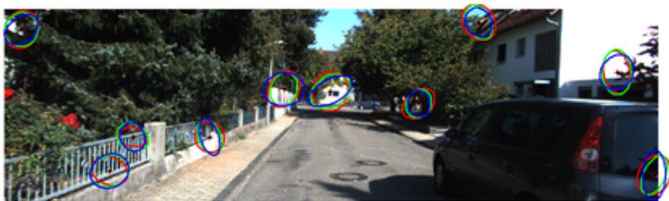
Fig. 5.4 Harris features with position uncertainties for each RGB channel visualised through error ellipses. Covariances from each channel is coloured according to the channel.
