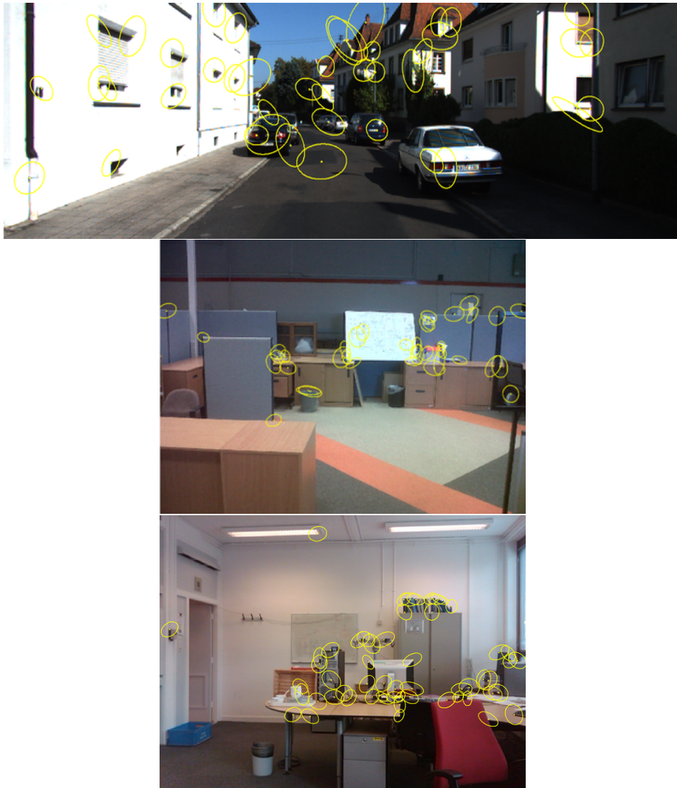
Fig. 5.3 Harris features with position uncertainties visualised through error ellipses.
