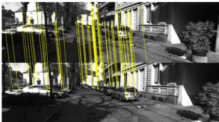
Fig. 4.7 Illustration of feature matching on sample of images used in motion estimation.
