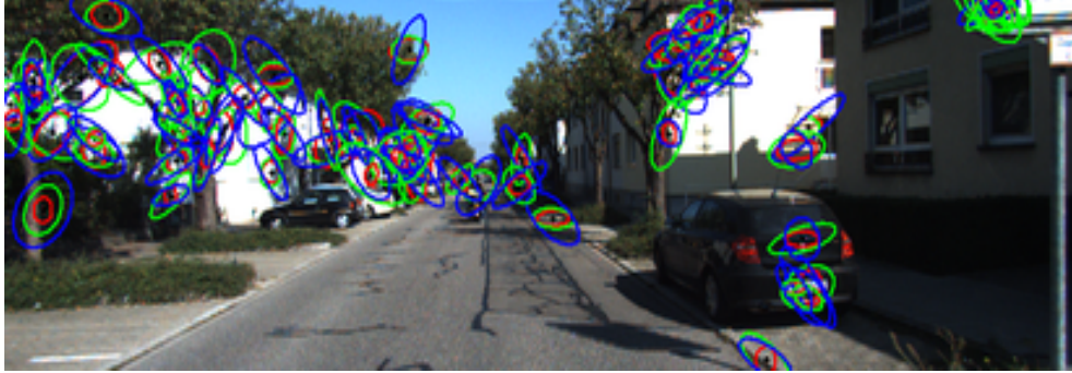
Fig. 5.6 SIFT features with position uncertainties for each RGB channel visualised through error ellipses. Covariances from each channel is coloured according to the channel.
