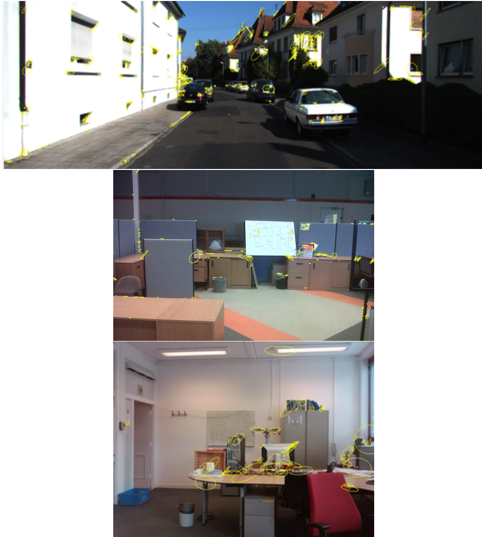
Fig. 5.5 SIFT features with position uncertainties visualised through error ellipses.
