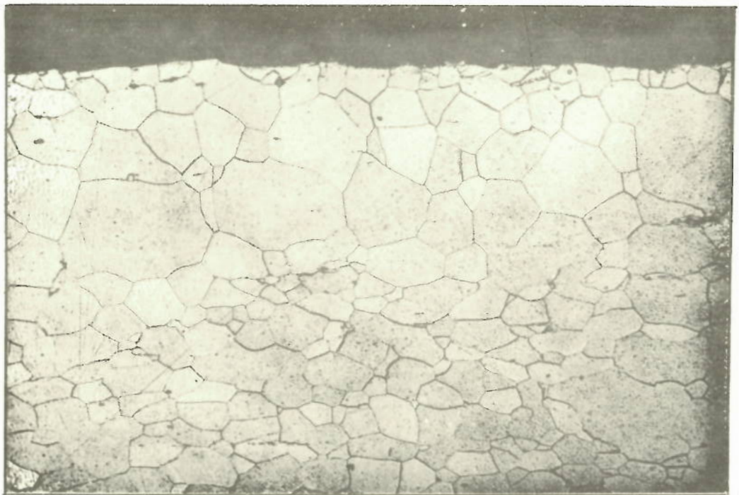
FIG. 6 ETCHED X 400 SHOWING EDGE → CENTRE GRAIN SIZE VARIATION
