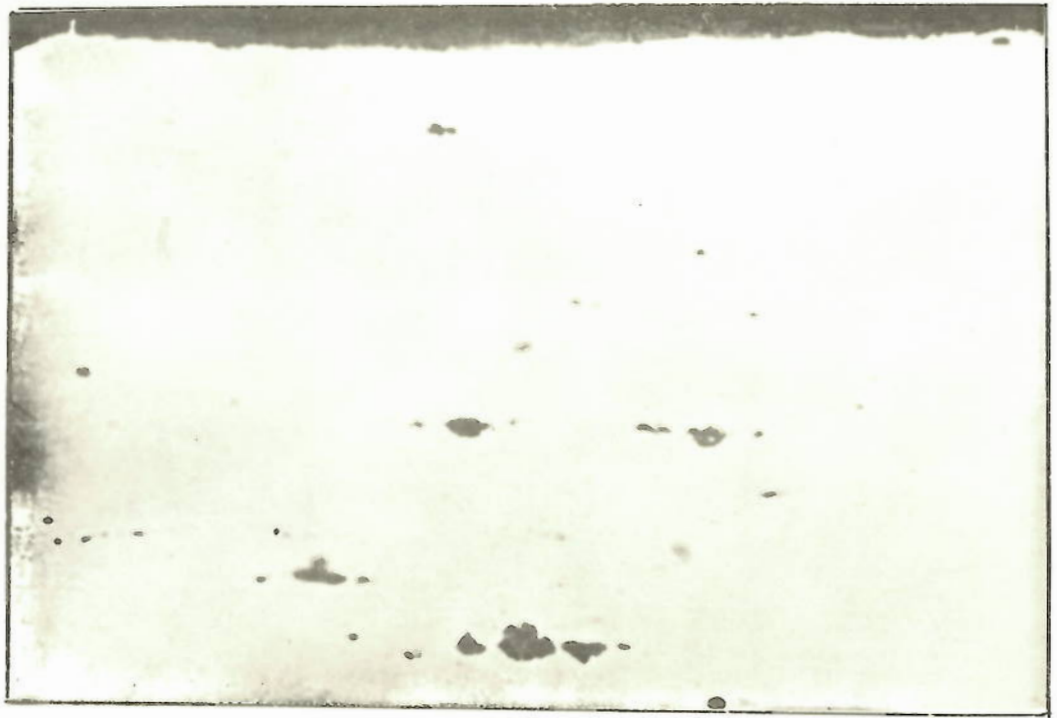
FIG. 5 UNETCHED X 400 SHOWING NON METALLIC INCLUSIONS
