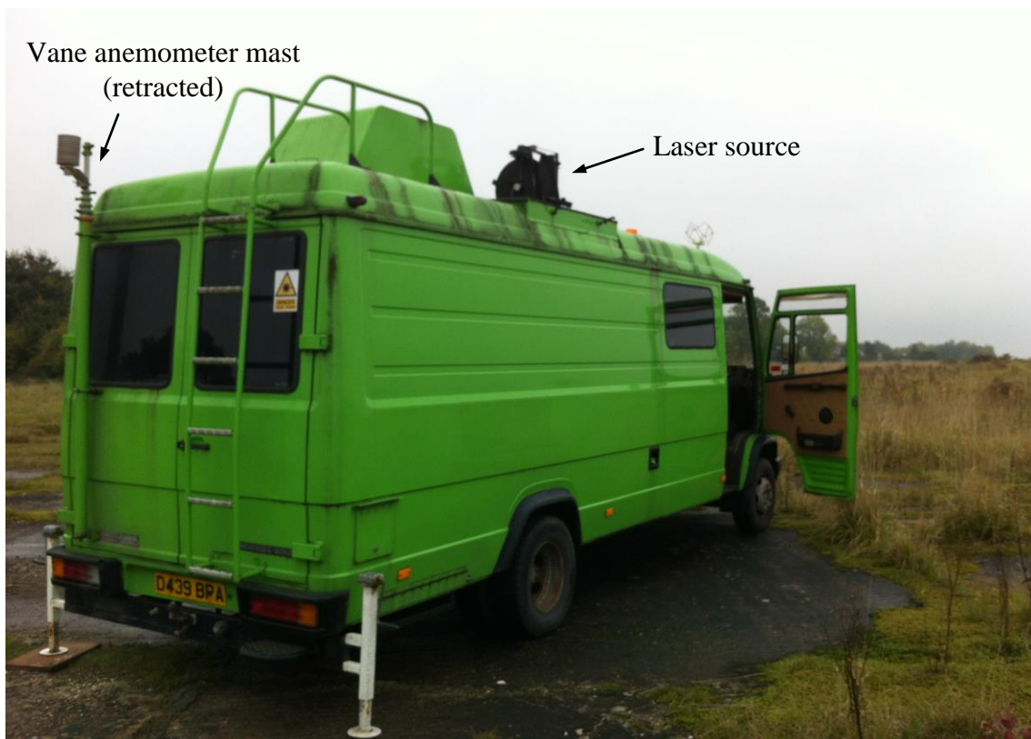
Figure H.3: Lidar vehicle used for plume dispersion measurements during the field trials at Cranfield Airport
