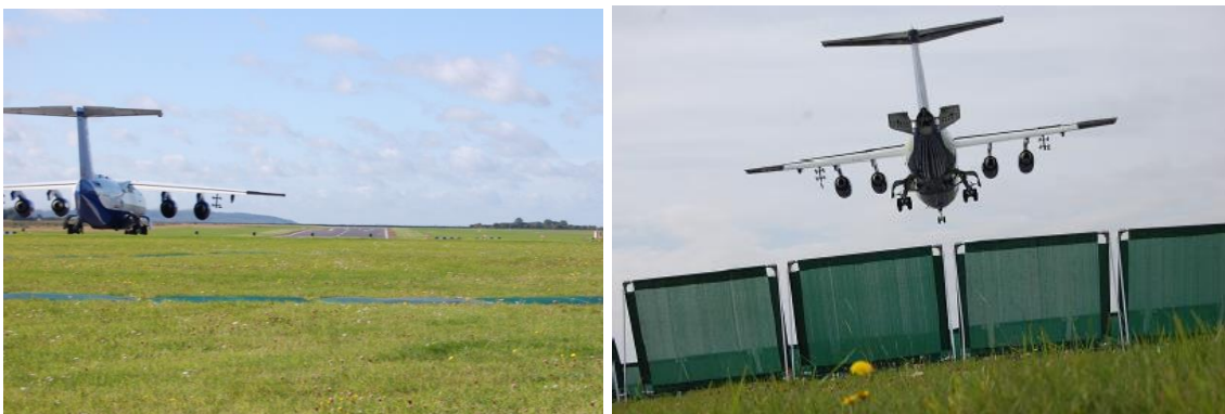
Figure 8.3: FAAM BAe 146-301 during field trials, September 2011: (a) starting take-off run, baffles deflated (image by Bennett, 2012), (b) during landing approach, baffles erected (image taken from Bennett et al., 2013)
