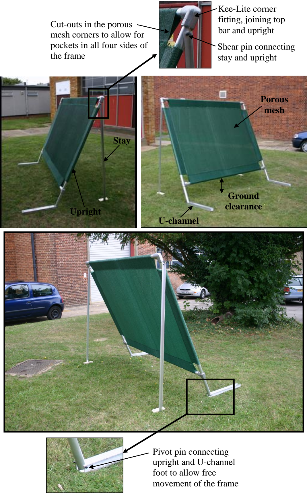
Figure 8.1: Design features of the baffle prototypes used in the field trials
