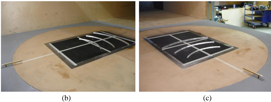
Figure 7.17: 8'x4' ABLWT working section arrangement for force balance measurements at 1:100 scale: a) schematic of Sortie 11 (top view, turntable not shown); b) image of Sortie 10 (isometric view, flow direction is from bottom left); c) image of Sortie 11 (isometric view, flow direction is from bottom right)
