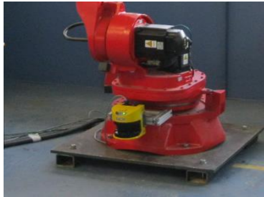
Figure 5-30 Single arm industrial robot (left) and the laser scanner (right)
