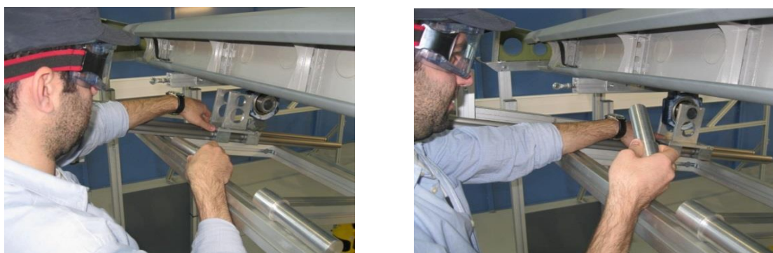
Figure 5-42 Alignment of the carriages to the sub-assembly's bearings (left) and securing them using a bearing pin (right)
