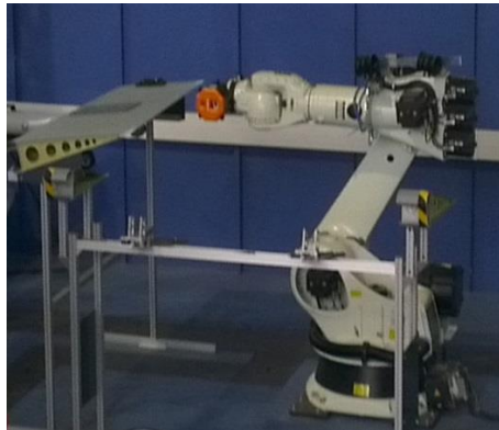
Figure 2-19 The human-robot collaborative demonstrator for aircraft equipping processes
