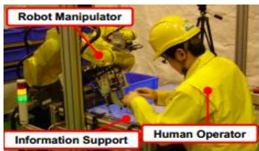
Figure 2-17 A human-robot collaborative system for a wiring operation (Retrieved from: Tan, Duan, Zhang, Watanabe, Kato and Arai, 2009)
