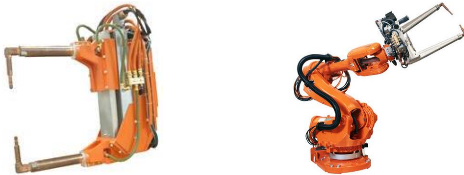
Figure 2-7 Example of a spot-welding tool (left) attached on an industrial robot (right) 5
