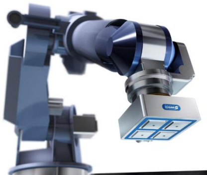
Figure 2-6 Example of magnetised grippers 4
