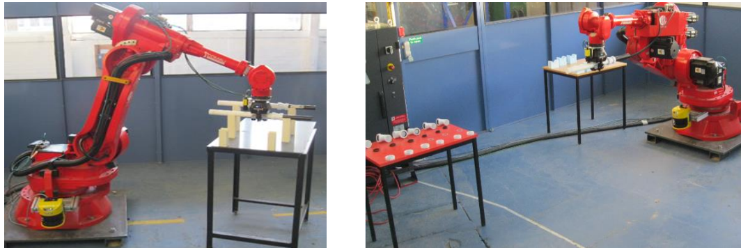
Figure 5-36 The robot picks-up the pipe (left) and positions it for assembly (right)
