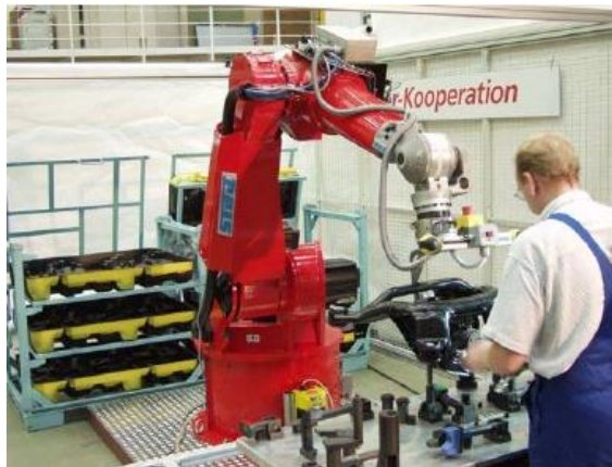
Figure 2-8 The PowerMate collaborative system (Retrieved from Schraft, Meyer, Parlitz and Helms, 2005)
