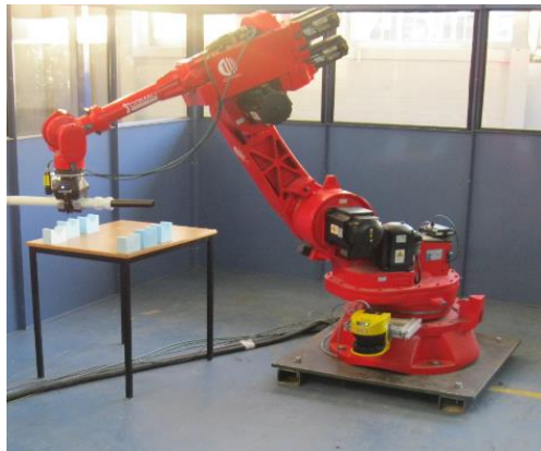
Figure 5-38 Drop-off position of the completed item
