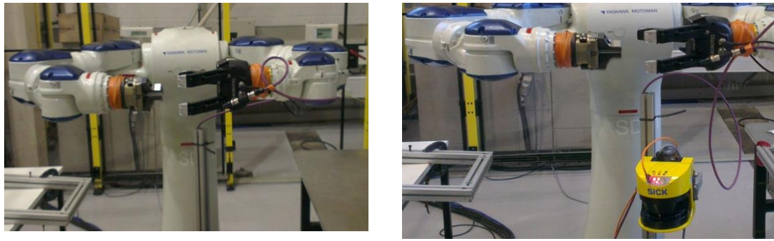
Figure 5-32 Twin arm industrial robot (left) and the laser scanner (right)
