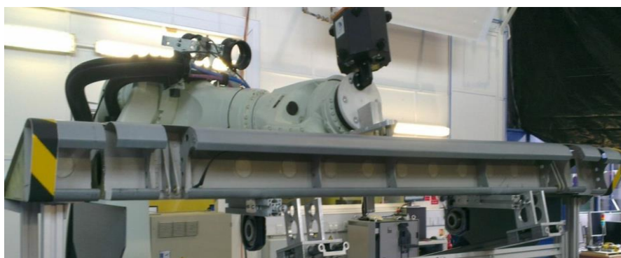
Figure 5-41 Positioning of the sub-assembly on the stand by the robot
