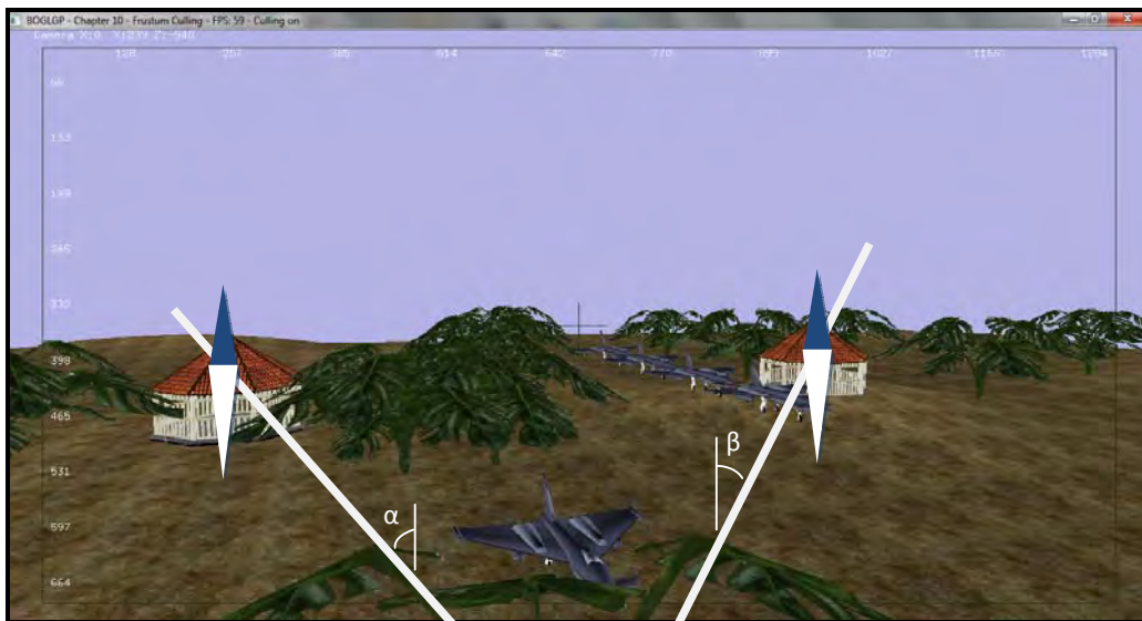
Figure 30: Determining the individual position by triangulation. North-south directions are indicated by the blue-white pointers. The angles \alpha and \beta as well as the positions of the houses are known.
