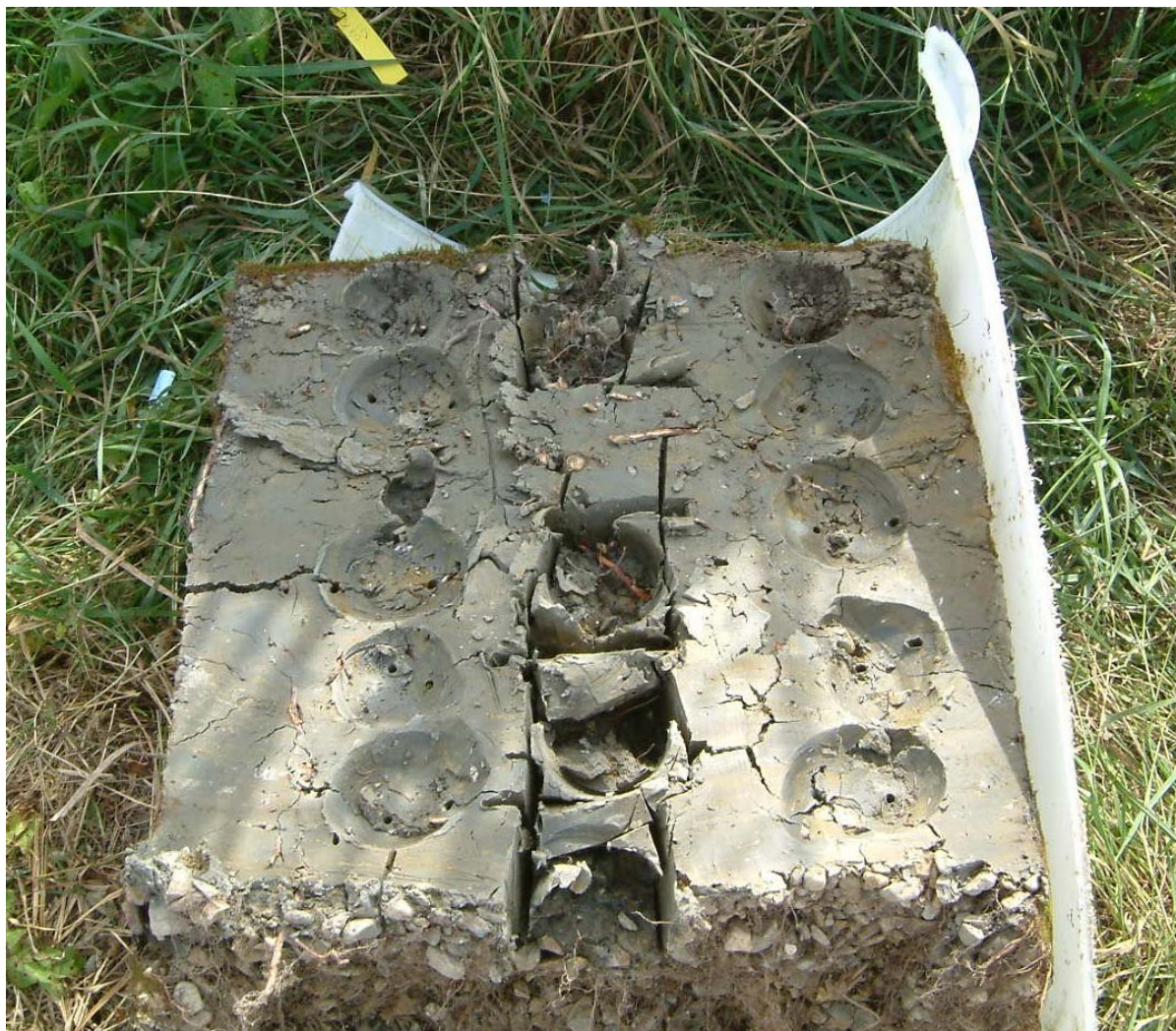
Figure 6.5: A broken up lysimeter, note the middle section (sample 2 for each zone is harvested for collection of soil for chemical analysis; note the polypropylene sheath around the lysimeter.
