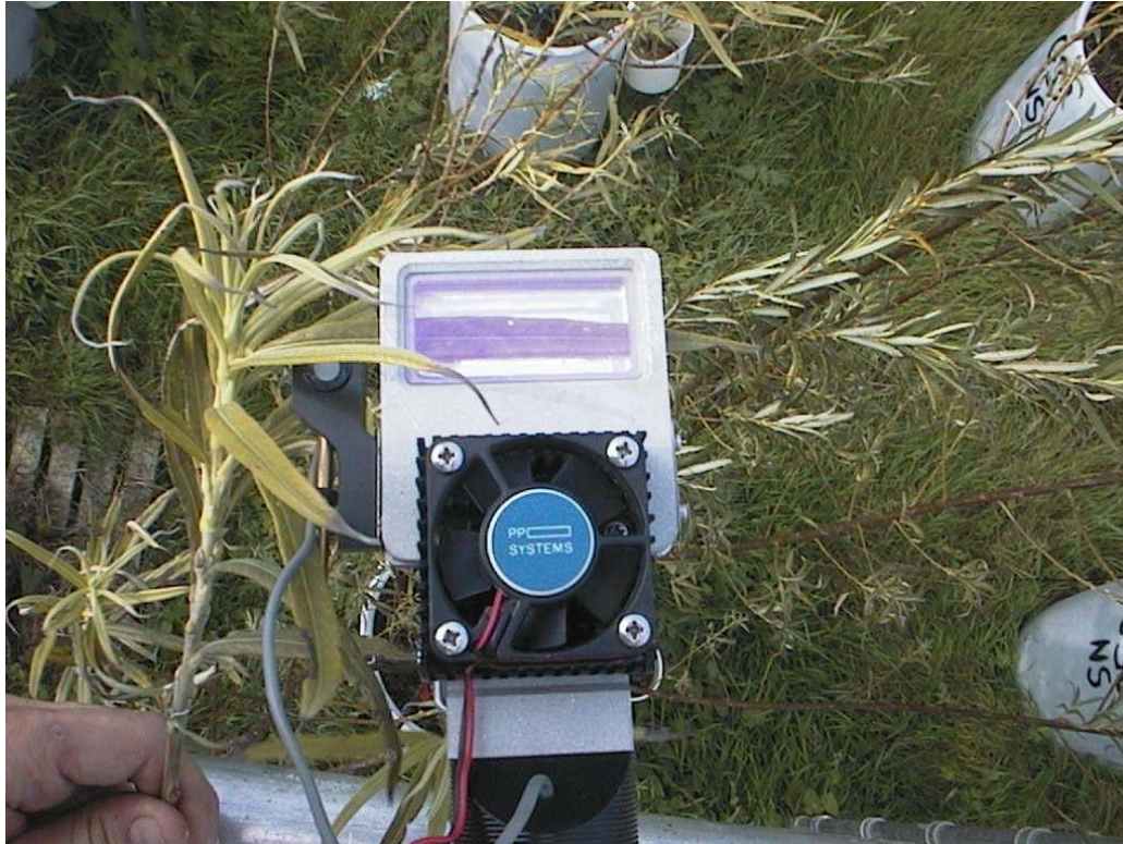
Figure 5.3: A leaf being held horizontally within the cuvette. Note that the leaf does not fill the cuvette chamber.
