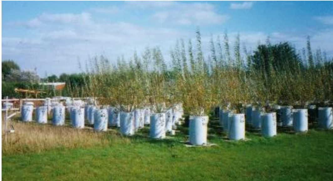
Figure 2.1: The experimental plot showing the lysimeters supporting one year old Salix viminalis (Cranfield University, Silsoe, Bedfordshire) in May 2001.
