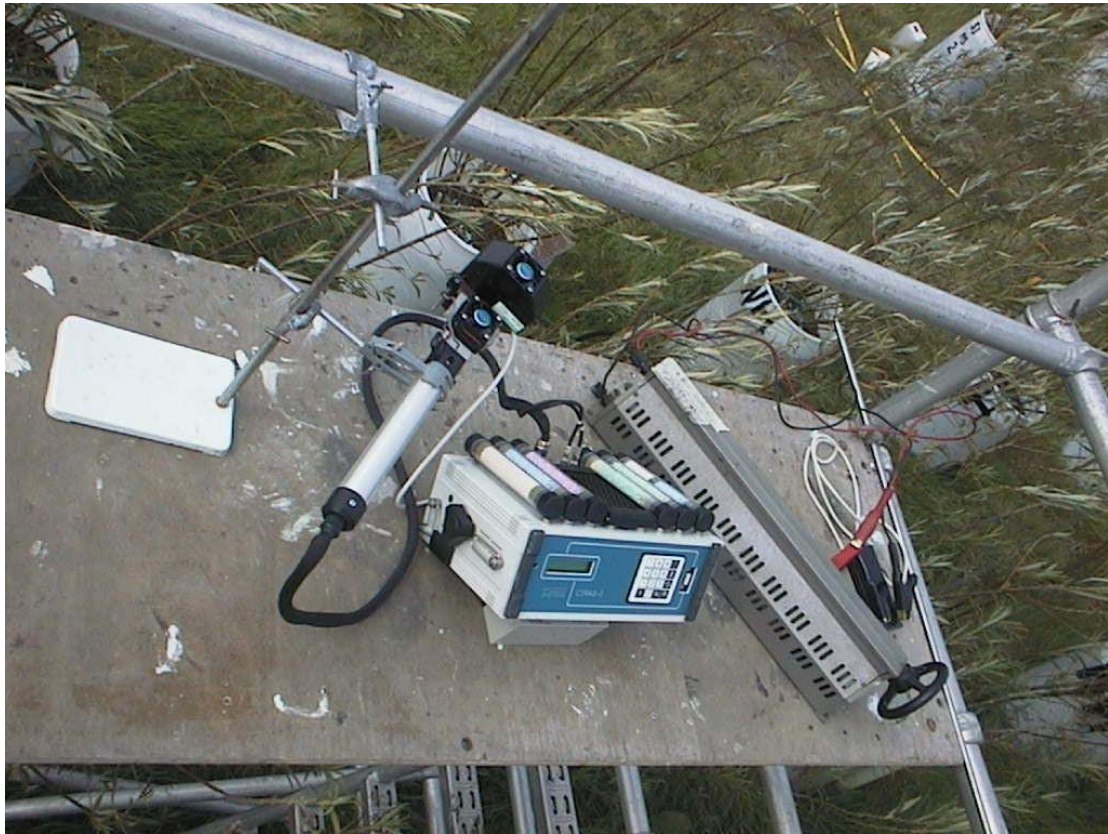
Figure 5.2: The CIRAS-1 on a platform tower set up to take measurements for a PAR curve, note the light source, clamp and variable resistor.
