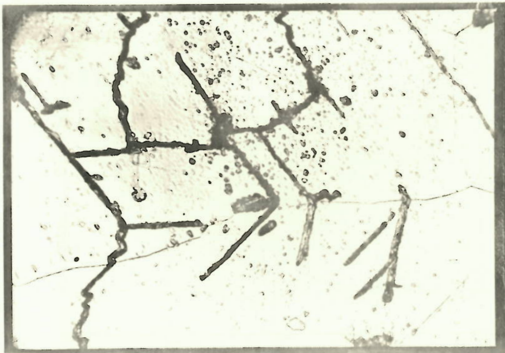
FIG. 22. Fatigue cracks in cladding.
