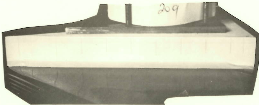
FIG. 20. 20^\circ WEDGE, \alpha = 3^\circ , UPPER SURFACE, CLEARANCE 0.010'' , M_{\infty} = 1.28
