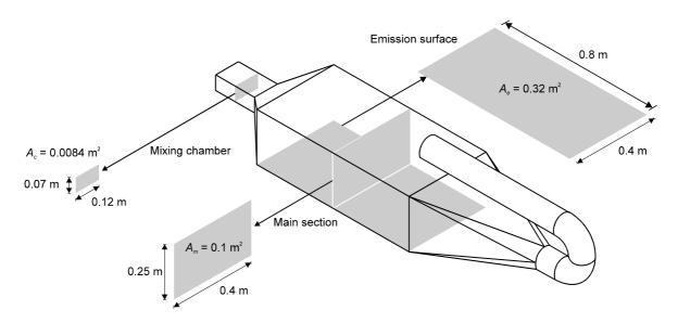
Figure 2 Schematic of wind tunnel and dimensions
