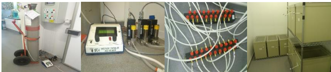
Figure 3.5 Schematic diagram of the ethylene supplementation setup
