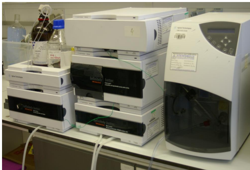
Figure 3.8 HPLC-ELSD system used to quantify sugars
