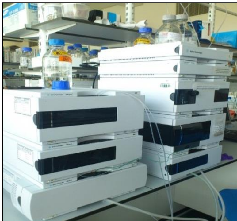
Figure 3.10 HPLC-DAD system used to quantify the phenolic compounds
