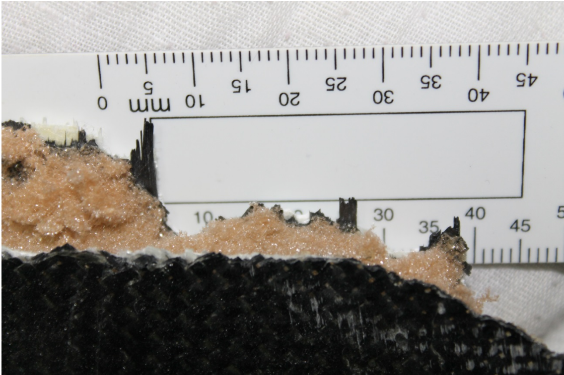
Figure 6-24 – Lower sandwich structure showing evidence of tensile failure. The orientation of the protruding fibres are 0^\circ (Source: Author)
