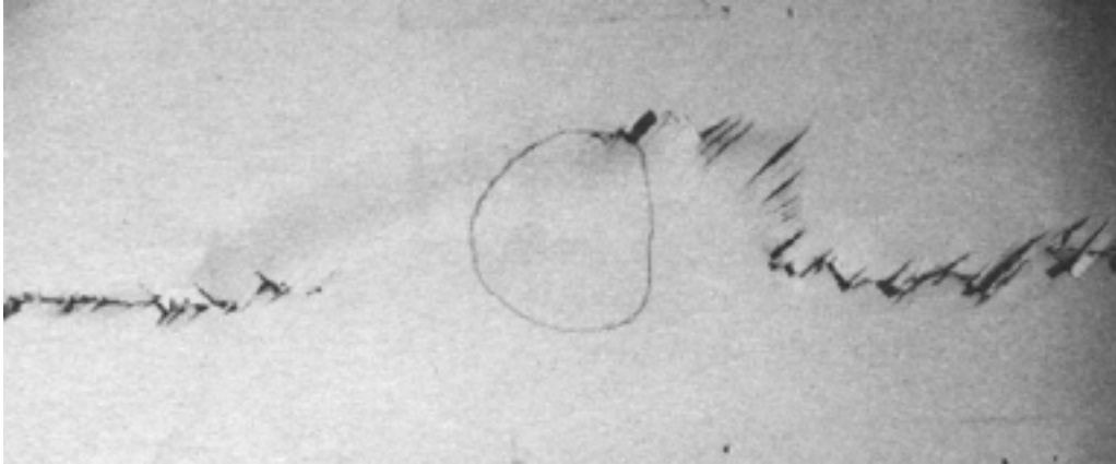
Figure 5-9 - Example of compression cracking in an impacted laminate (Greenhalgh & Cox, 1992)
