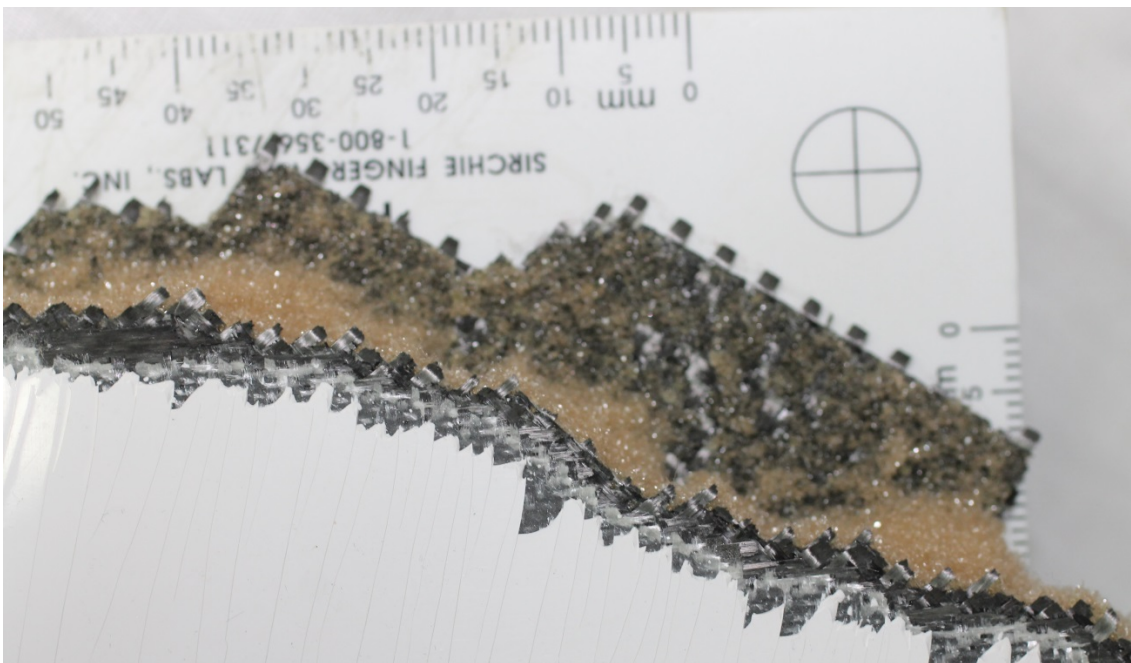
Figure 6-23 – Lower sandwich structure from the right wing illustrating fibre pullout. The orientation of the protruding fibres are \pm 45^\circ (Source: Author)
