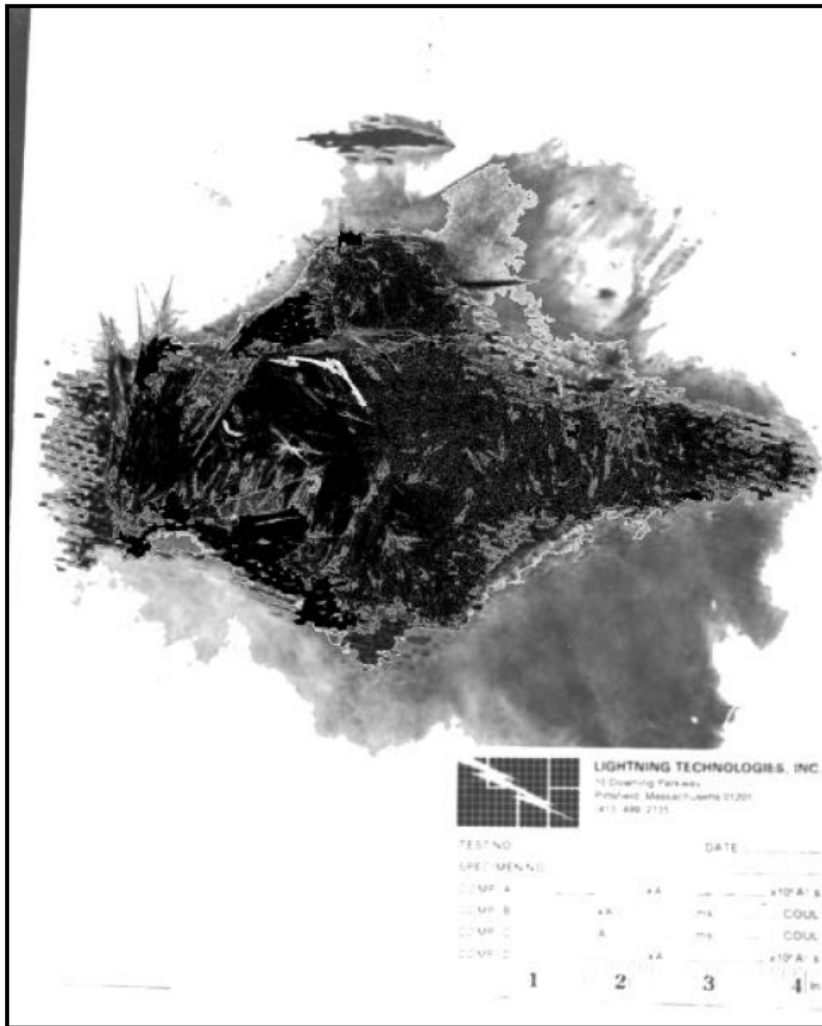
Figure 5-27 – Zone 1A strike to a painted exterior surface of unprotected 4 ply 0.052 in. CFC laminate of woven cloth (Rupke, 2002)
