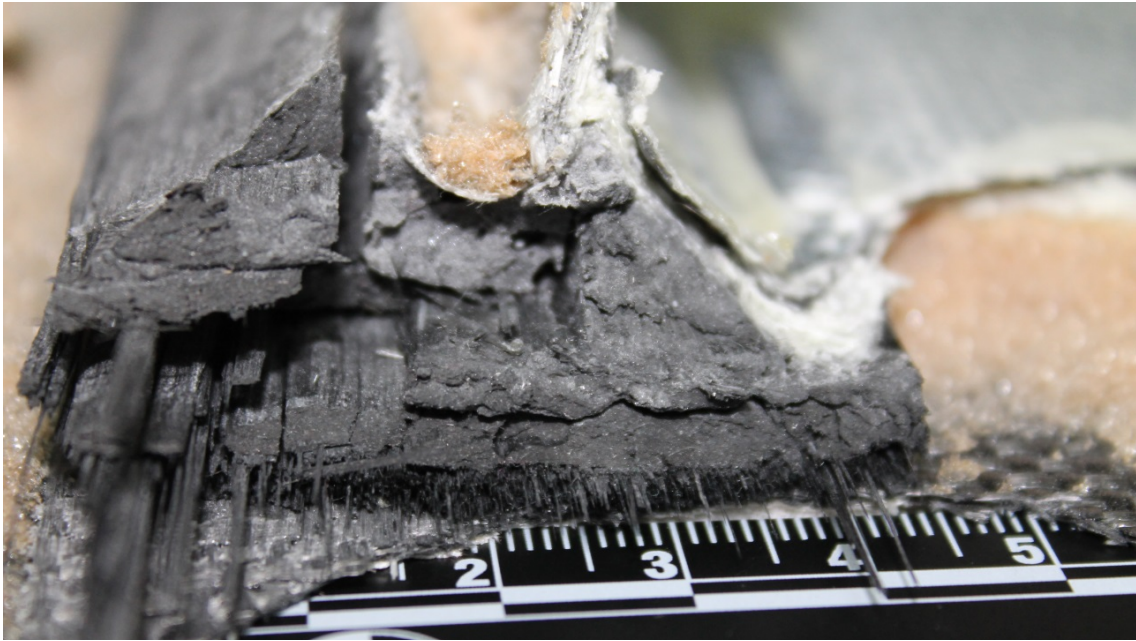
Figure 6-21 – Lower spar cap from the left wing showing characteristics of flexural failure. Note the compressive fracture surface (Source: Author)
