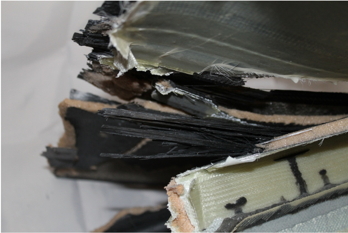
Figure 6-45 – Deformation of the upper spar cap from the right wing (Source: Author)
