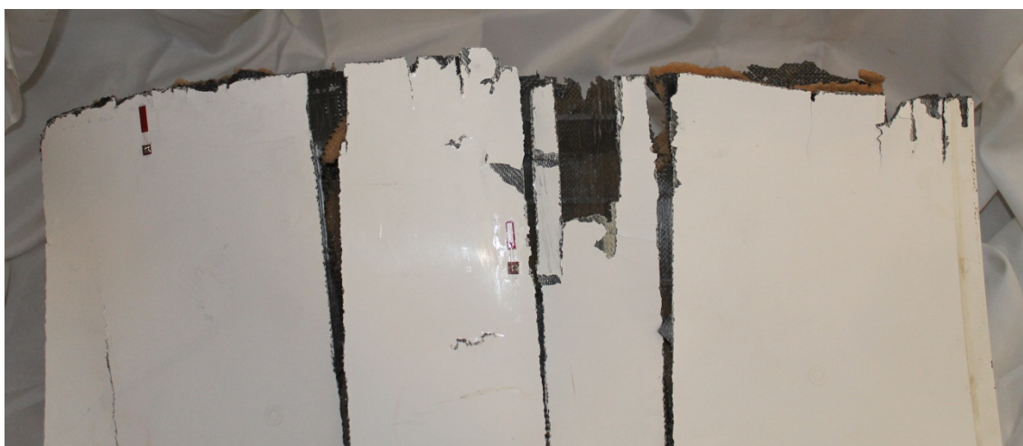
Figure 6-38 – Right wing upper surface. The impact location can be identified as a semi-circular fracture deviation on the top centre of the image (Source: Author)
