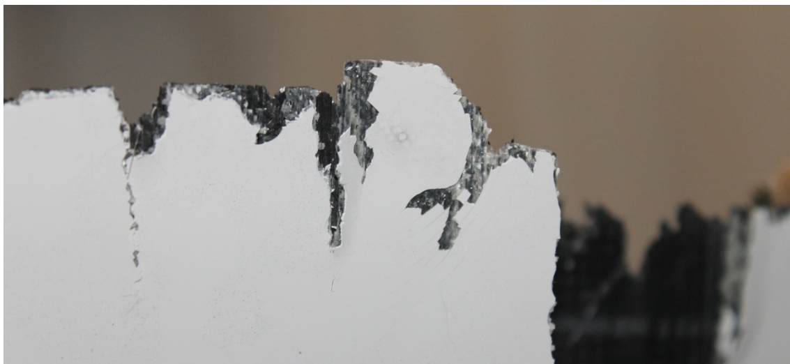
Figure 6-37 – Deflection of the translaminar fracture induced by the impact (Source: Author)
