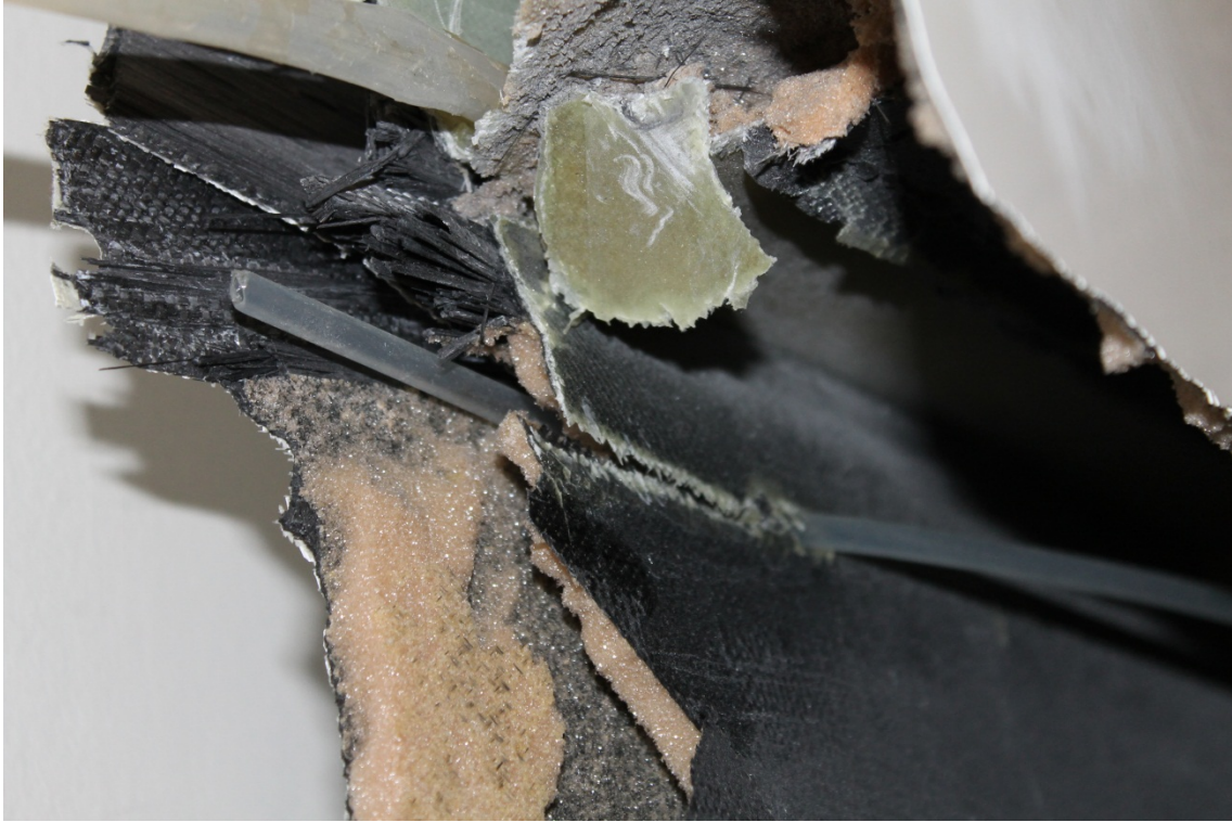
Figure 6-46 – Pull through of a polymer tube inducing fracture of the upper skin lower laminate (Source: Author)
