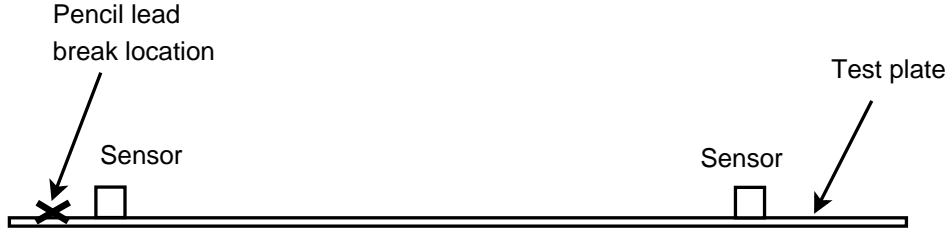
Figure 4.1: Setup for determining propagation velocity of AE signals in 2mm thick 2014 T6 aluminium plates
