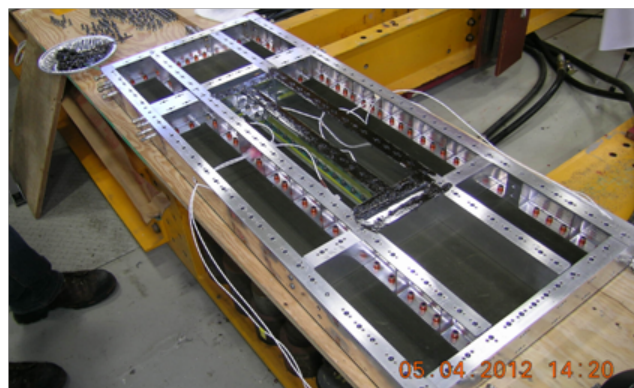
Figure 3.17: Network of spars and ribs in wing-box
