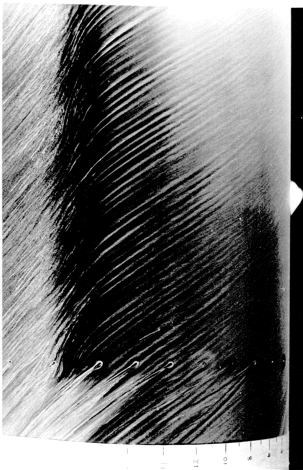
Frontispiece - A surface oil flow pattern showing a transition to turbulence which is produced by a sweep induced instability of the laminar boundary layer.
