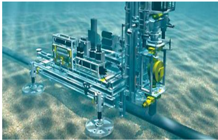
Figure 1-4: Remote Hot Tap Cutting machine as used for the Asgard B Gas Compression Project 139
