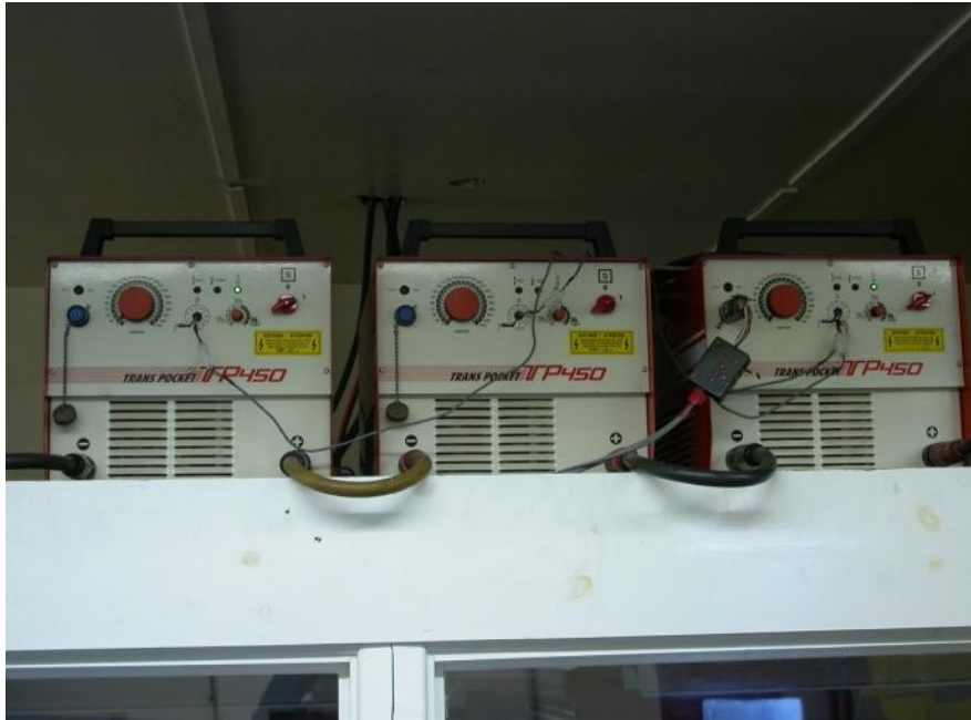
Figure 3-2: Fronius Trans Pocket TP 450 power sources in series
