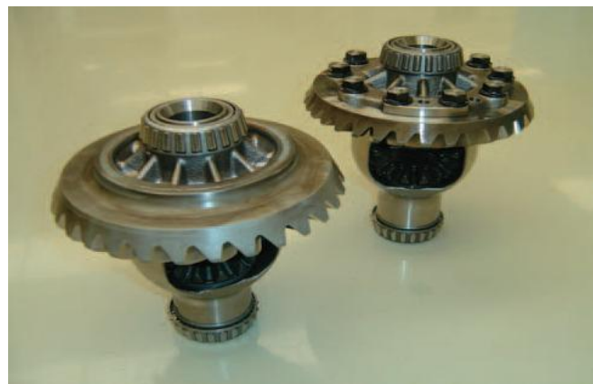
Figure 2-42: Welded (right) and bolted (left) differential gear sets
