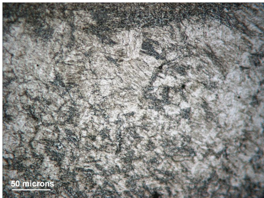
Figure 3-23:Microstructures of (top) penetration area and (bottom) heat affected zone from sections marked on the macrographs (insert) for the weld made at 100 bar with 8 m/min WFS and 7 mm/s welding speed
