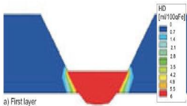
Figure 2-31: Hydrogen distribution after welding, HAZ gets significant hydrogen only near the melt line 65
