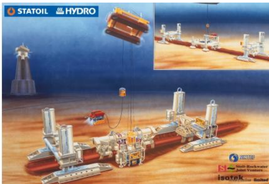
Figure 2-18: Illustration of the Pipeline Repair System spread at the seabed 156
