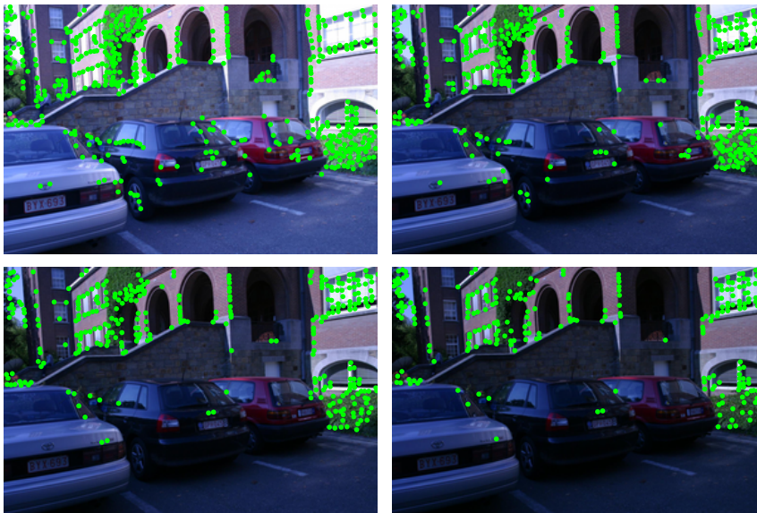
Figure 3.4: Harris Corners detection, Leuven sequence. Sequence to test invariance against illumination changes. Green dots represent the detected corners, namely, the pixels with a cornerness value higher than 10^8 , for k = 0.04 .
