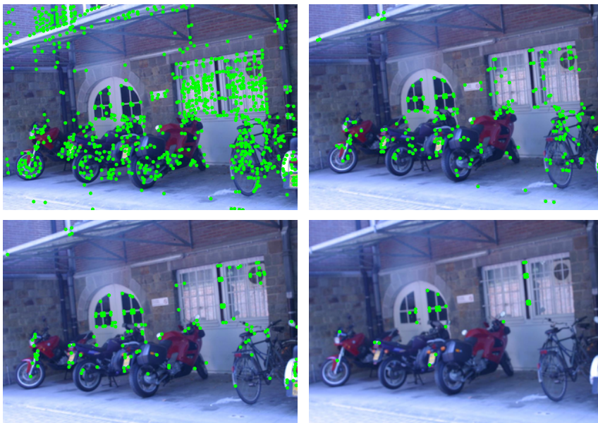
Figure 3.2: Harris Corners detection, Bikes sequence. Sequence to test invariance against blurring. Green dots represent the detected corners, namely, the pixels with a cornerness value higher than 10^7 , for k = 0.04 . A total of 846, 254, 147 and 35 corners are respectively detected.
