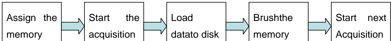
Figure 10-8: shows the single thread software procedure
