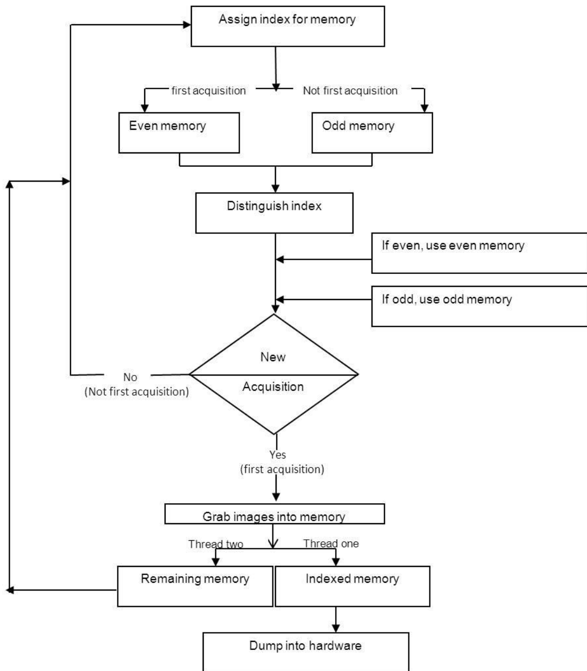
Figure 10-9: gives the flowchart of multi-threading configuration of MSI imaging system
