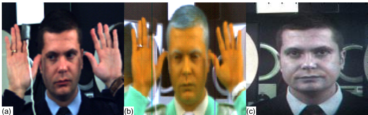
Figure 10-3: Shows the typical 'composite' images collected by the three spectral cameras (a) VNIR HSI (b) SWIR HSI (c) AOTF MSI using the acquisition software established by the author.
