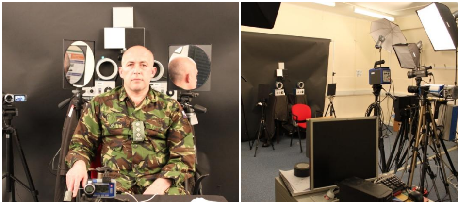
Figure 3-5. (Left): shows the layout of the experimental setup for the anxiety assessment exhibiting a range of calibration panels and black bodies in the background. The room is well illuminated (~750 lux) by diffused halogen lamps as shown in the picture on the right.
