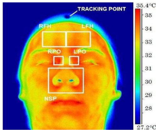
Figure 4-21 Features extracted from multiple ROI for arousal classification: left supraorbital (LFH), right supraorbital (RFH), left periorbital (LPO), right periorbital (RPO), and nasal (NSP) (Nhan BR., 2009).
