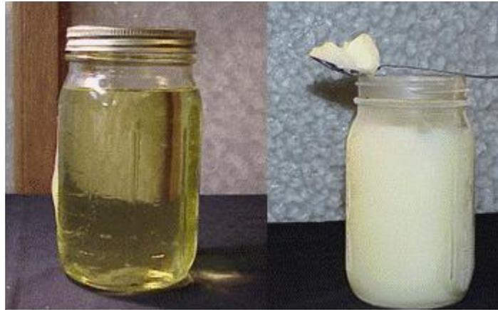
**Figure 1-4: The Tendency of Biodiesel to Freeze at Cold Temperature (Melanie, 2006)**
